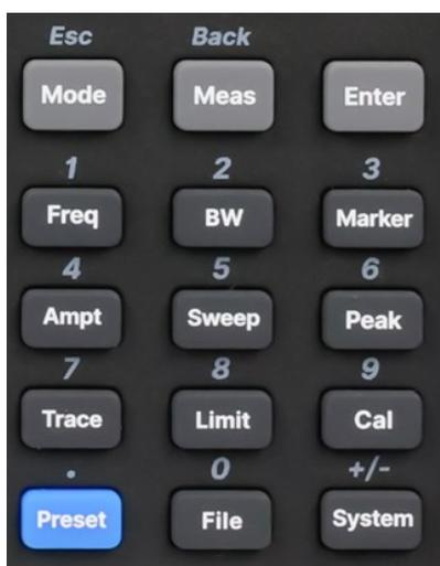
The function key part of the front panel is the reuse key of menu selection mode and value input mode, which can be switched by **Enter** and **Esc** :
