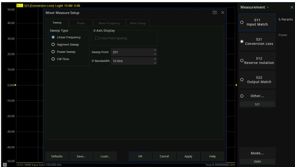
If the “show setup dialog” checkbox is unchecked, the Mixer Measure Setup dialog box will not pop up simultaneously when the user opens the mixer measurement function. If the user needs to modify the mixer parameter settings again, they can access the Mixer Measure Setup dialog box by pressing the front panel excitation condition buttons **【Start】 / 【Stop】 / 【Freq】 / 【Power】 / 【Sweep】** > mixer measurement.
