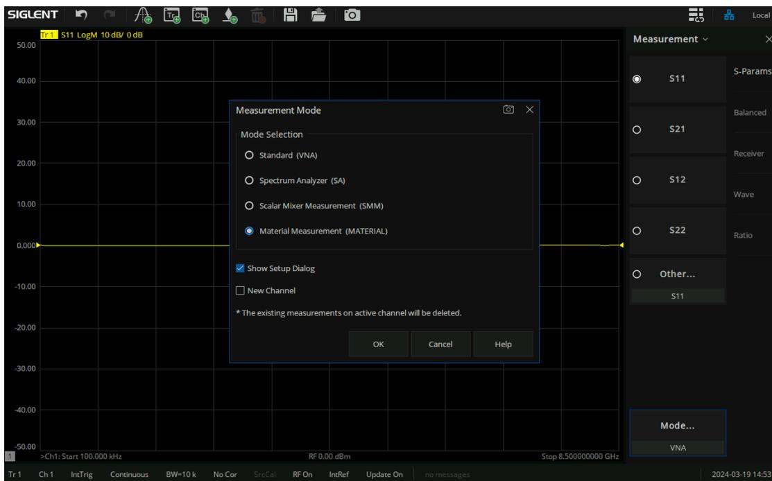
Figure 15-2 MATERIAL mode channel selection dialog box
