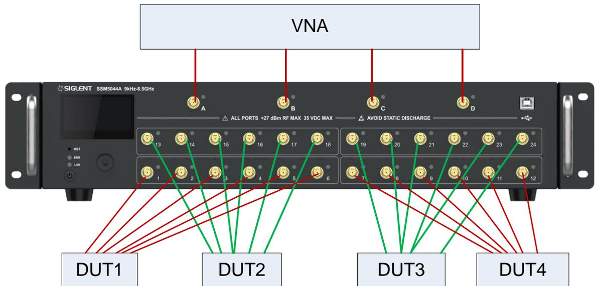
VNA and switch matrix combined expansion port diagram
