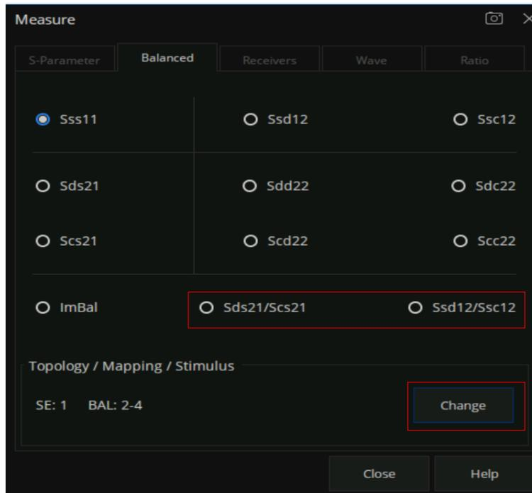
The table below shows the CMRR parameters available when measuring different balanced device.
