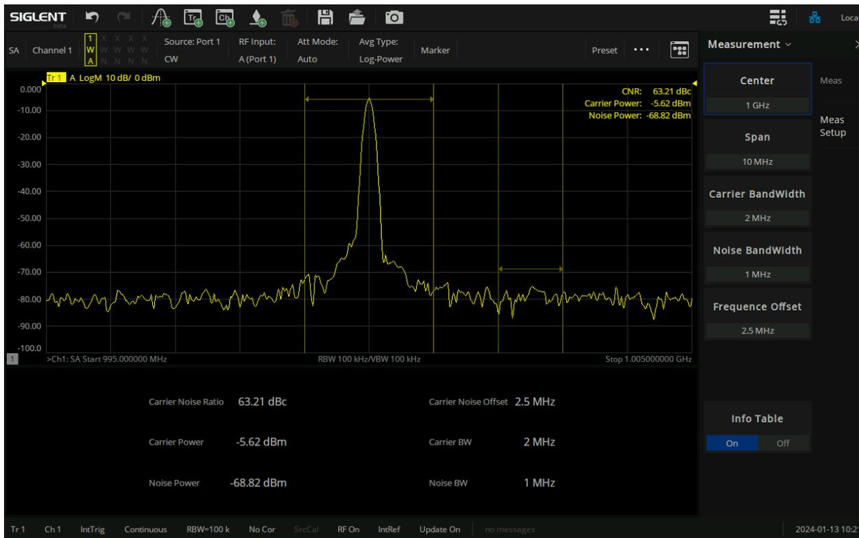
Figure 11-17 CNR measurement
