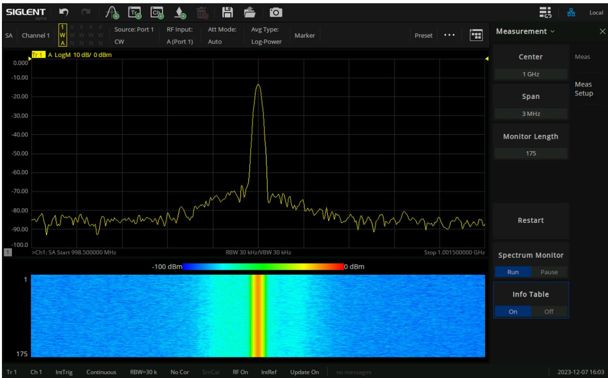
Figure 11-18 Spectrum Monitor
