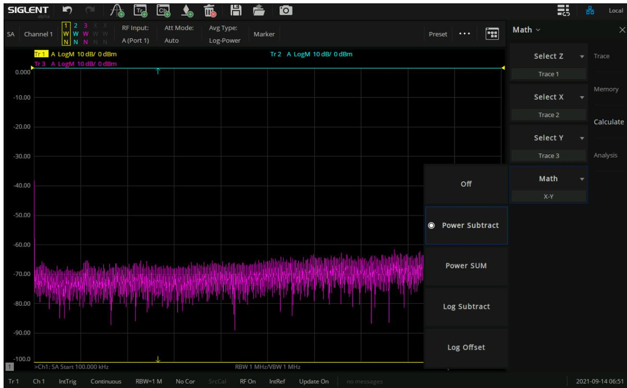
In the function expression  $z=f(x, y)$ , two identical input traces can be set, but the output trace cannot be set as the input trace at the same time. The input and output settings in different mathematical relationships are independent of each other. VNA provides four types of mathematical budgeting in SA mode:
