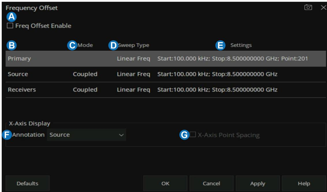
**A. Frequency Offset (ON/OFF)** Enables Frequency Offset Mode on ALL measurements that are present in the active channel. When frequency offset function is not enabled, all frequencies are the same as the Primary frequency.
