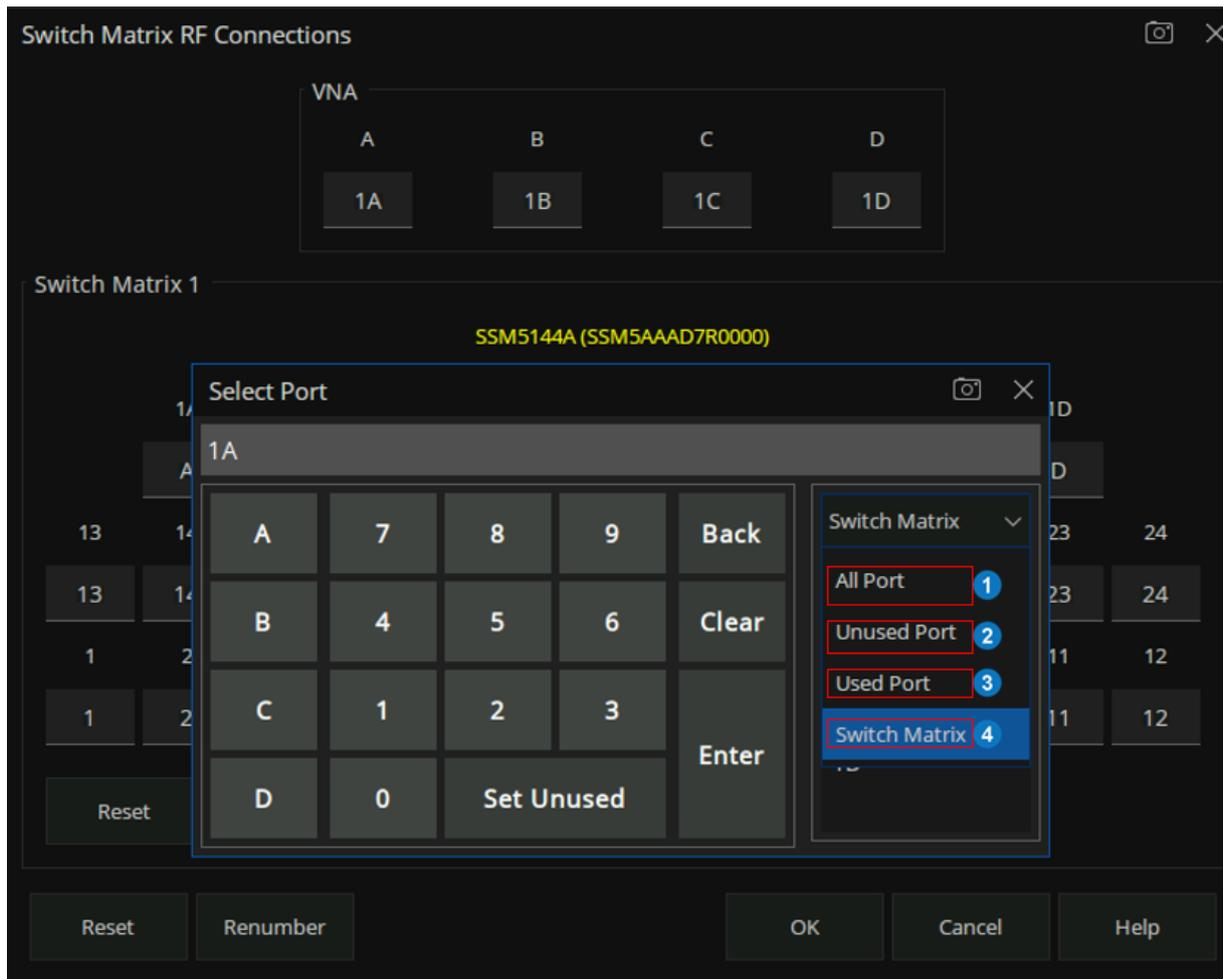
① **All Port:** Indicates all RF ports (including VNA RF ports and SSM RF ports). You can select a port from the drop-down list.
