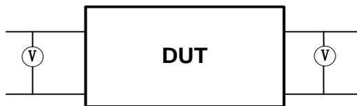
Fig 2-2 Balanced devices
