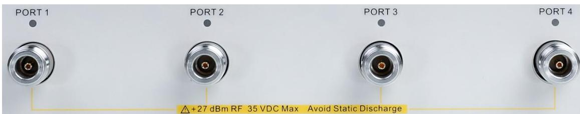
Figure 5-6 Front panel RF connectors (4-port VNA)
