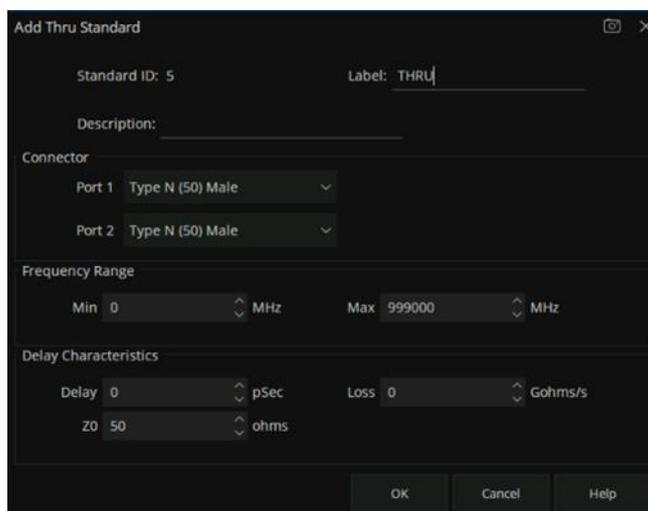
Figure 7-17 THRU Characteristics
