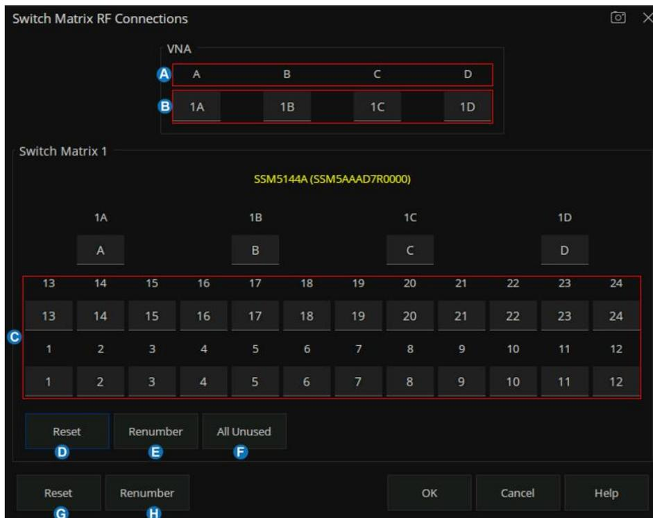
**A**: The A/B/C/D labels in the VNA check box indicate the four physical ports of the vector network analyzer port.
