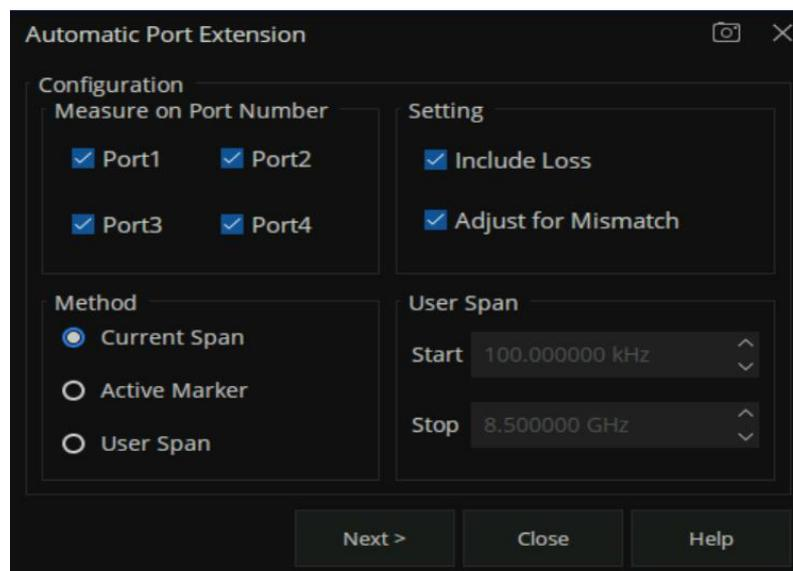
Figure 7-6 Automatic port extension setting interface
