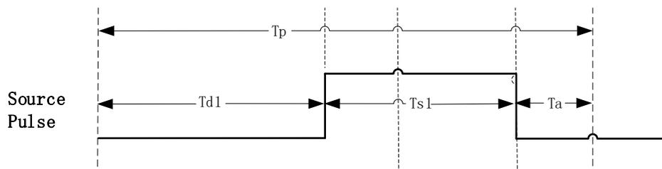
**Pulse Width:** Sets the width of the source pulse ( $T_{s1}$ ).
