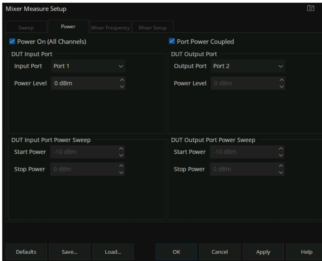
**Power On(All Channels):** Select to open all internal RF sources of VNA channels.
