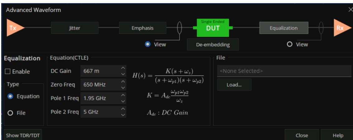
Figure 10-10-18 Equalization setting
