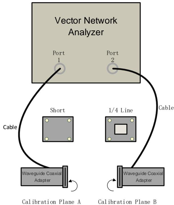
Figure 15-11 Schematic Diagram of Waveguide Calibration Connection
