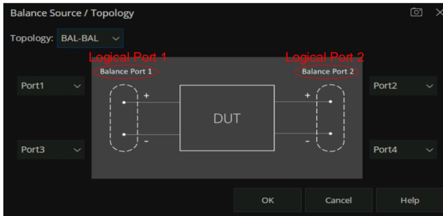
“Logical Port” is used to describe a physical analyzer test port that has been remapped to a new port number.
