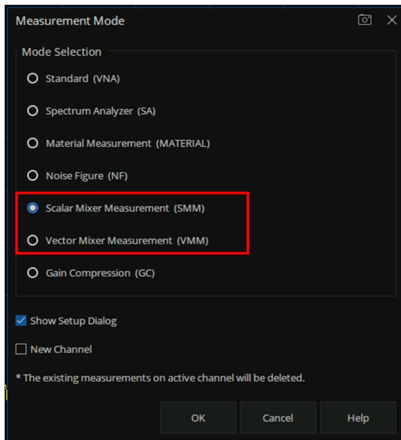
The "show setup dialog" checkbox is selected by default, indicating that every time the mixer is turned on for measurement, a Mixer Measure Setup dialog box will pop up for users to set mixer related parameters, as shown in the following figure.
