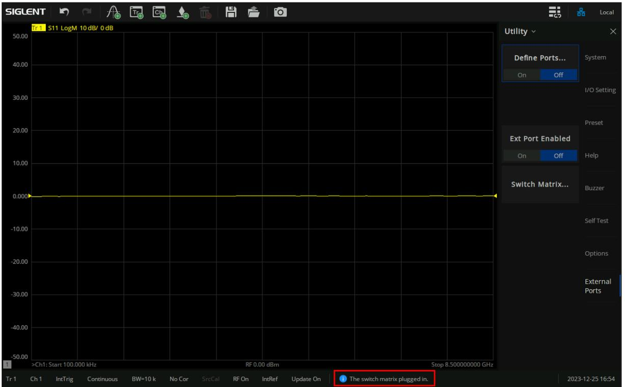
2. Press the **System** > **External Ports** > **Ext Port Enabled** to enable the function, then the matrix identifier
