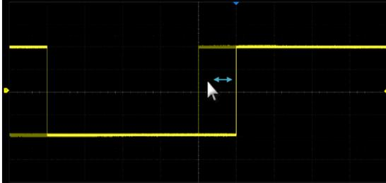
Click-and-drag the waveform left and right to move it on the horizontal axis
