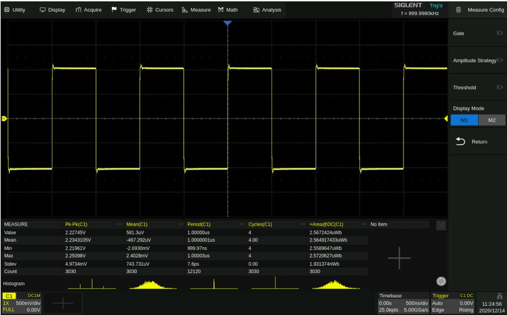
In M2 mode, up to 12 parameter measurements are displayed at a time. When statistics are enabled, they are distributed on the right side of the measurement item. Click a row to add or replace a measurement.
