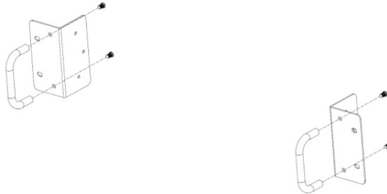
2. Install the rack flanges to the instrument using six M3×6 screws.
