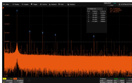
Hardware-accelerated FFT supports up to 8 Mpts operation. This provides high-frequency resolution with a fast refresh rate. The FFT function also supports a variety of window functions so that it can adapt to different spectrum measurement needs. Three modes (Normal, Average, and Max hold) can satisfy different requirements for observing the power spectrum. Auto peak detection and markers are supported.
