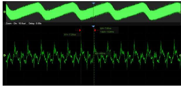
Using a hardware-based Zoom technique and record length of up to 500 Mpts, users can select a slower timebase without compromising the sample rate, and then quickly zoom in to focus on the area of interest.
