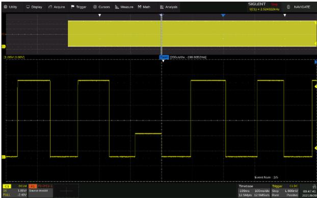
The oscilloscope can search events specified by the user in a frame. Events flagged by the Search can be recalled automatically using Navigate. It can also navigate by time (delay position) and history frames.
