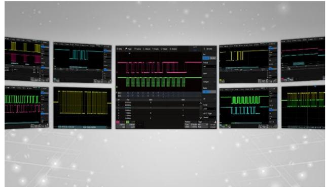
Display the decoded characters through the events list. Bus protocol information can be quickly and intuitively displayed in tabular form. I<sup>2</sup>C, SPI, UART, CAN, LIN, CAN FD, FlexRay, I<sup>2</sup>S, MIL-STD-1553B, SENT, and Manchester are supported.
