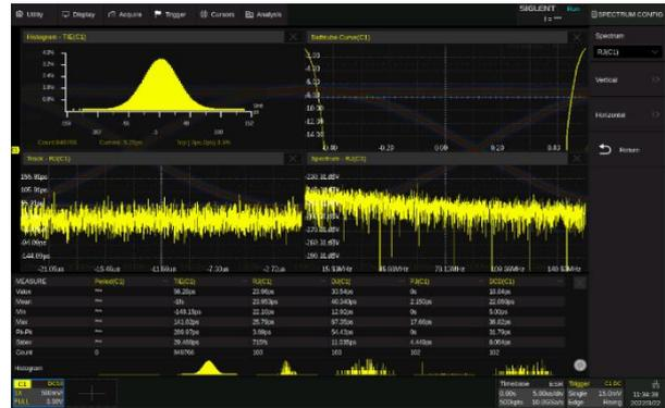
Supports eye diagram and jitter analysis / measurement. It can automatically extract the embedded reference clock from serial data and create an eye diagram. Measurement on multiple eye / jitter parameters is provided and mask testing of eye diagrams is supported.
