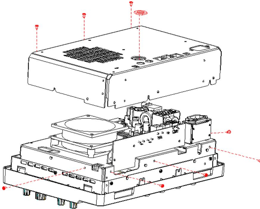
Figure 13 To remove the rear metal cover
