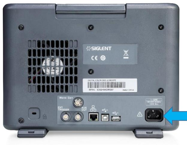
Figure 1 Connect the power cord
