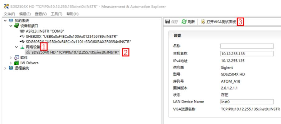
5. Click “ Open VISA Test Panel ” option button, which then displays the following interface ( below ). Then click the “ Input/Output ” option button and click the “ Query ” option button. The “ Read ” operation information will be displayed.
