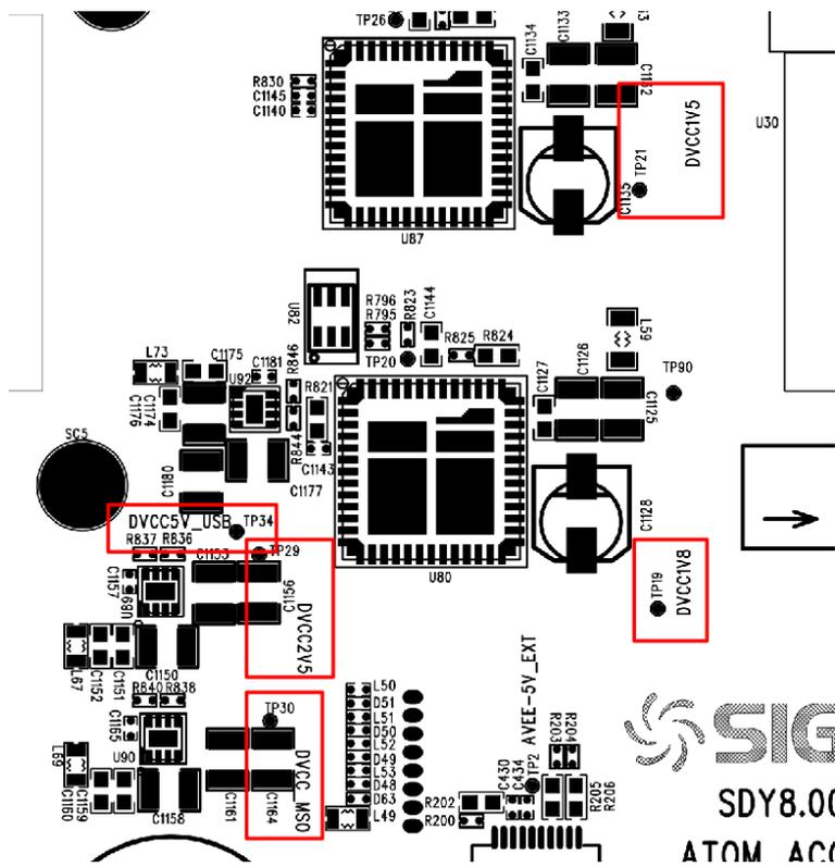
Figure 20 Test points for the Acquisition board power supplies (continued)
