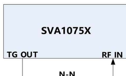
Figure 3-10 Connecting test instruments for TG Output
