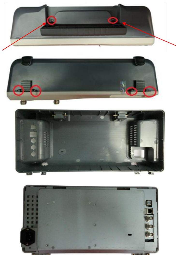
Figure 4-1 Removing the Rear Panel Screws
