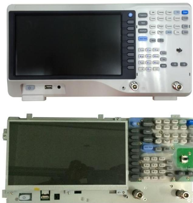
Figure 4-2 Removing the front panel
