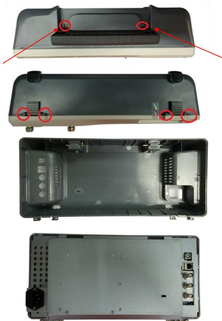
Figure 4-1 Removing the Rear Panel Screws
