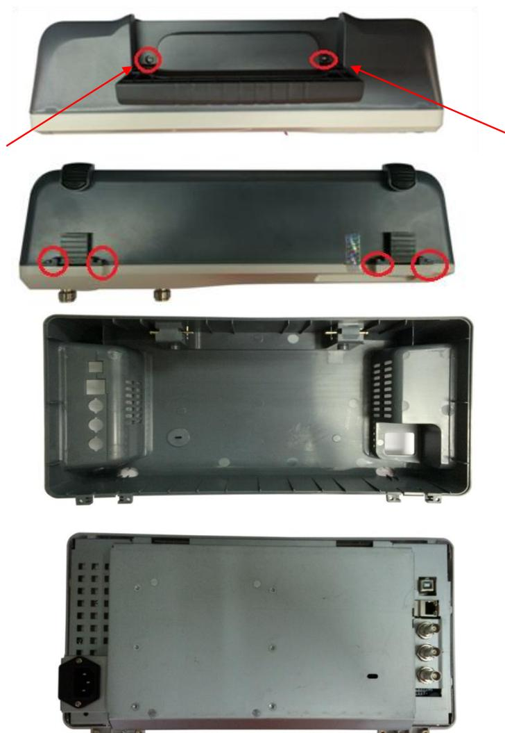
Figure 4-1 Removing the Rear Panel Screws
