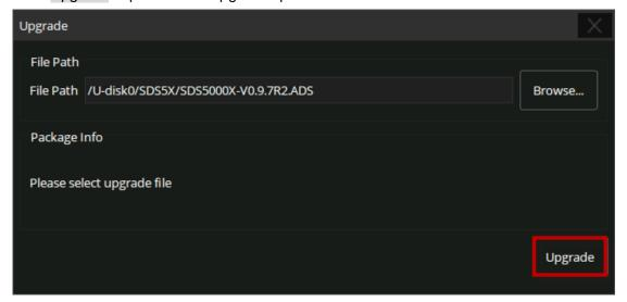
The system will first copy and verify the upgrade package. After the upgrade package
