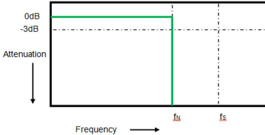
In fact, digital signals have frequency components above the fundamental frequency (a square wave is composed of a sine wave of the fundamental frequency and numerous odd harmonics), and generally, for oscilloscopes with a bandwidth of 500 MHz and below, the system has a Gaussian frequency response.
