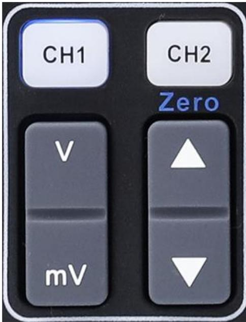
**CH1** : Analog input channels. The two channels are marked by different colors which are also used to mark both the corresponding waveforms on the screen and the channel input connectors.
