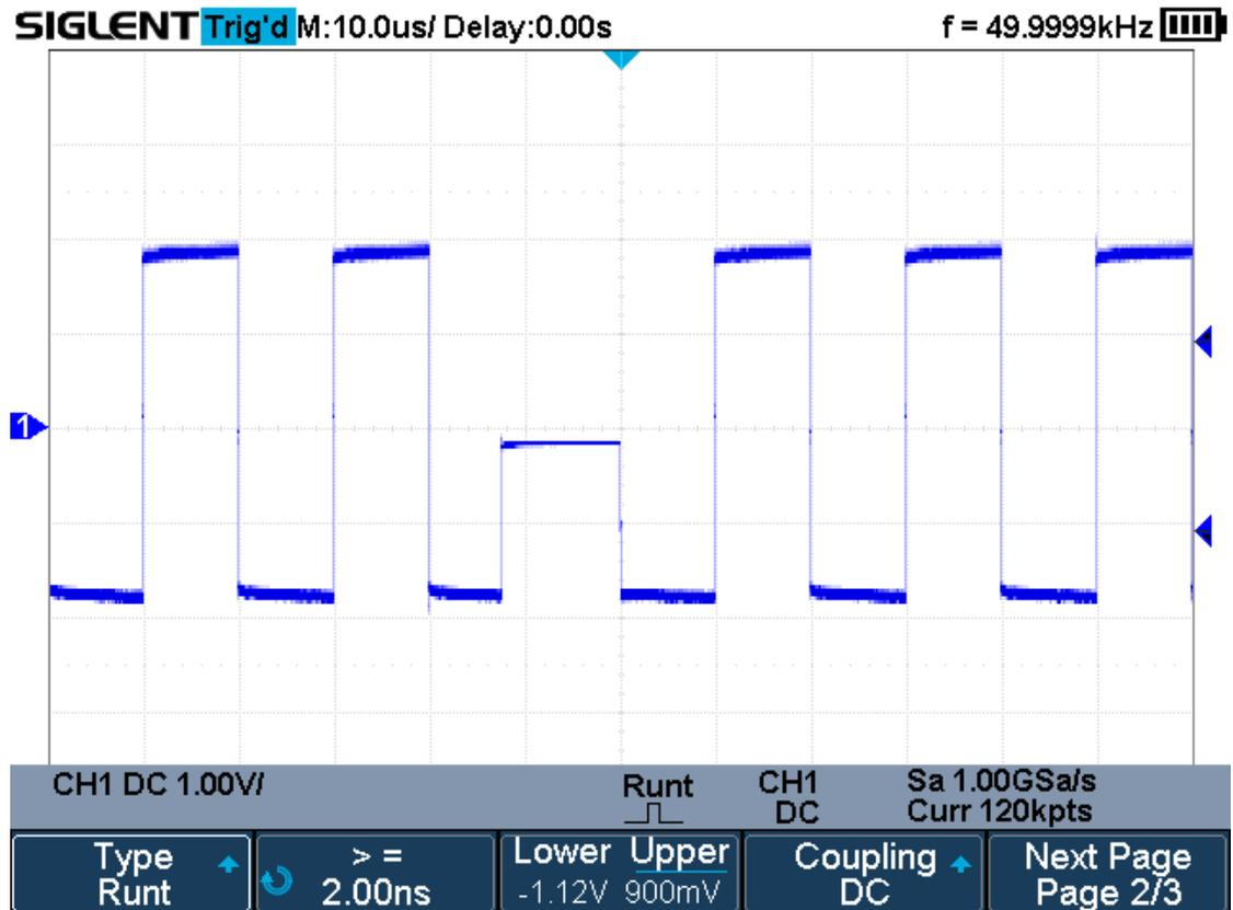
Figure 36 Runt Trigger
