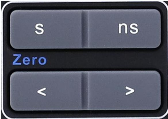
**Horizontal Position Button:** adjust horizontal position. Press the button to change the horizontal delay time, waveforms of all channels will move horizontally with the trigger point. Press the **Shift** + **Horizontal Position** to quickly reset the horizontal delay to Zero.
