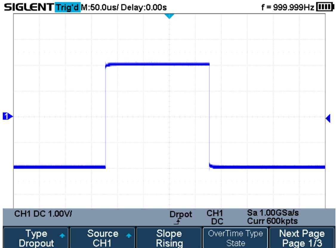
Figure 35 State Dropout Trigger
