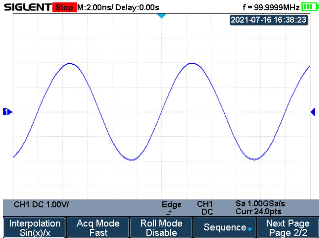
Figure 17 Sinx/x Interpolation
