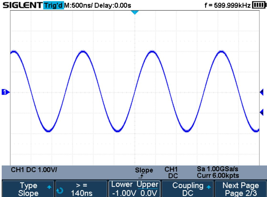
Figure 28 Slope Trigger
