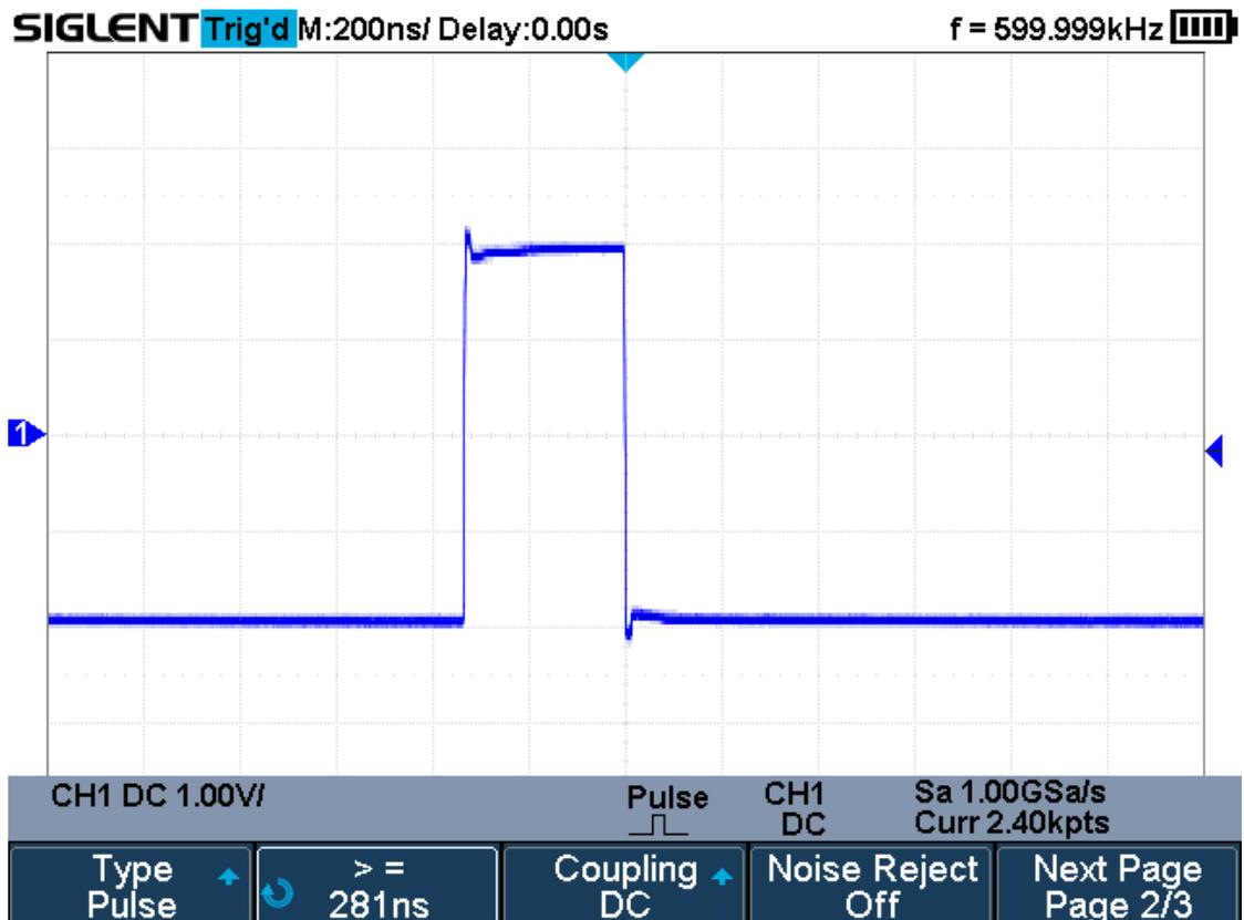
Figure 29 Pulse Trigger
