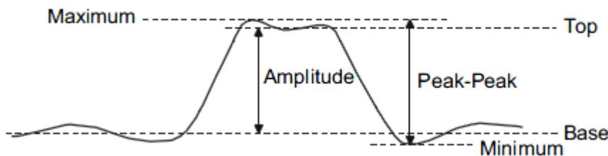
Figure 78 Voltage Measurements
