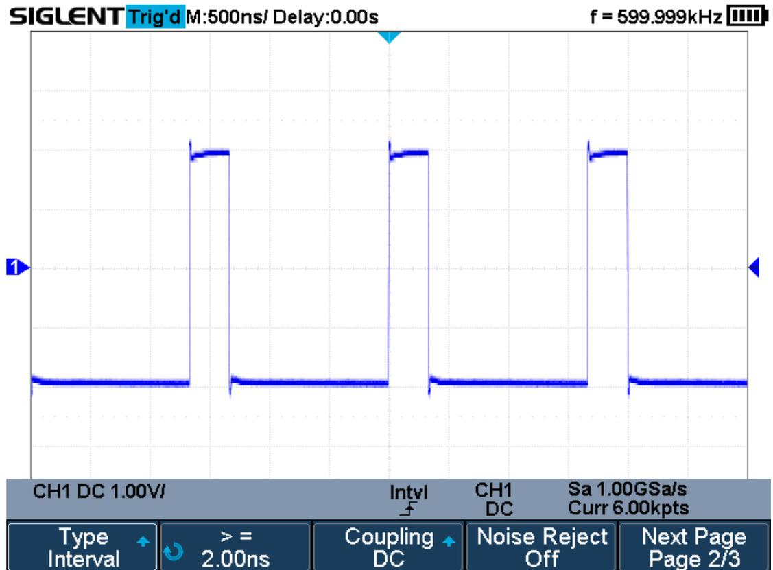
Figure 33 Interval Trigger
