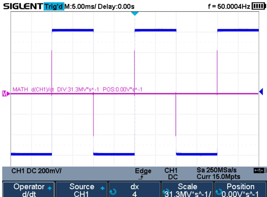
Figure 73 Difference Function Operation
