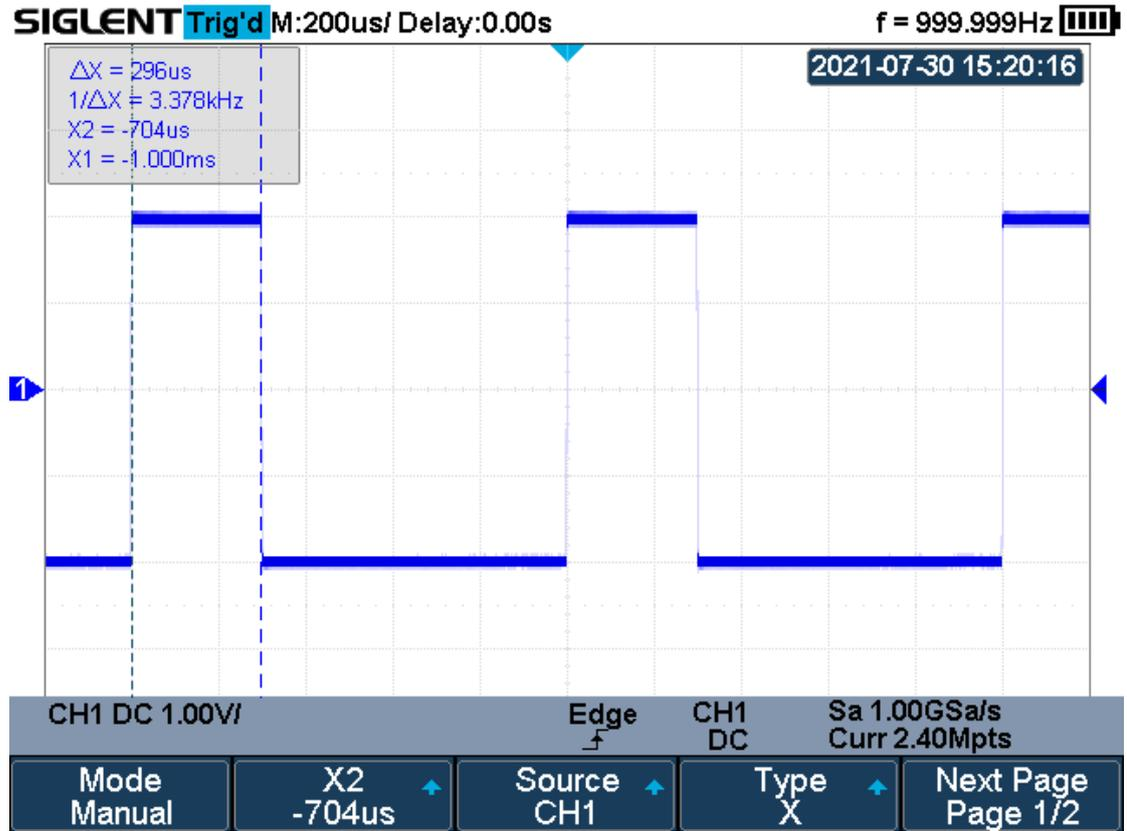
Figure 77 Measure Pulse Width
