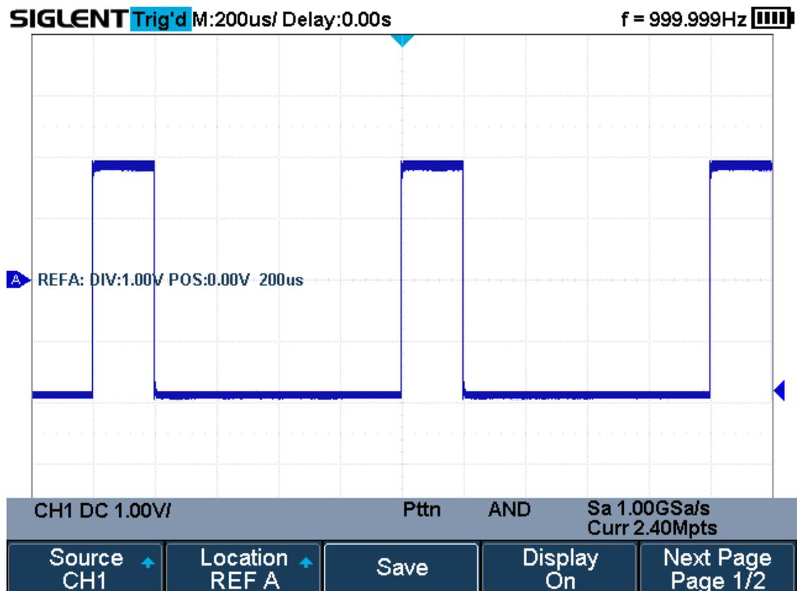
Figure 61 Reference Waveform
