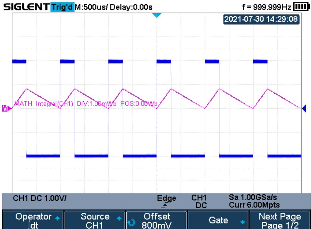
Figure 75 Integral with Offset
