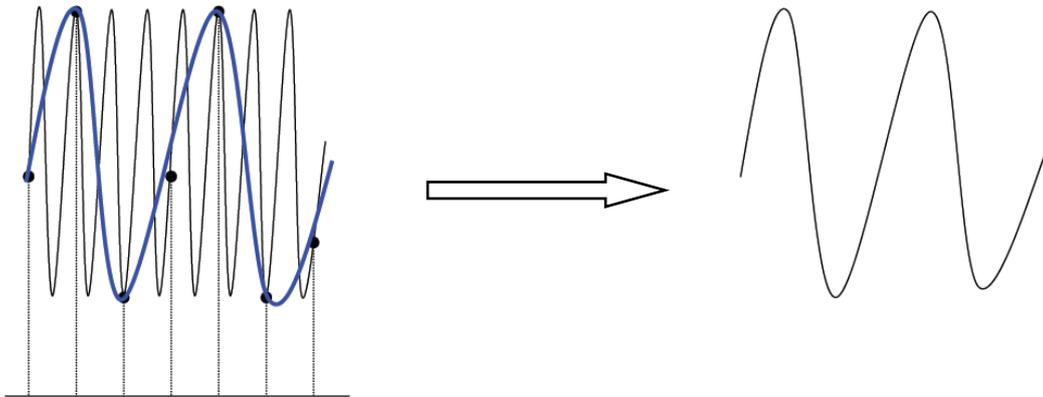
3. **Waveform Leakage:** when the sample rate is too low, the waveform reconstructed from the sample data cannot reflect all the actual signal information.
