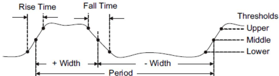
Figure 81 Time Measurements
