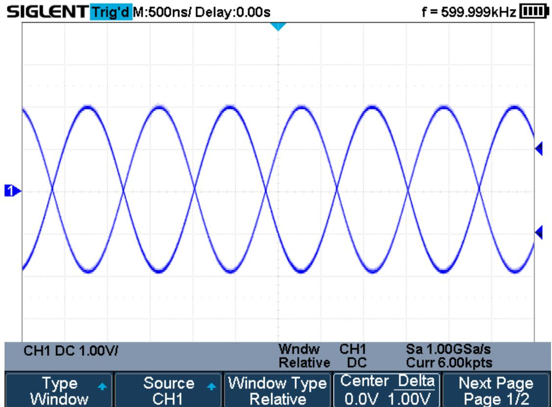
Figure 32 Relative Window Trigger
