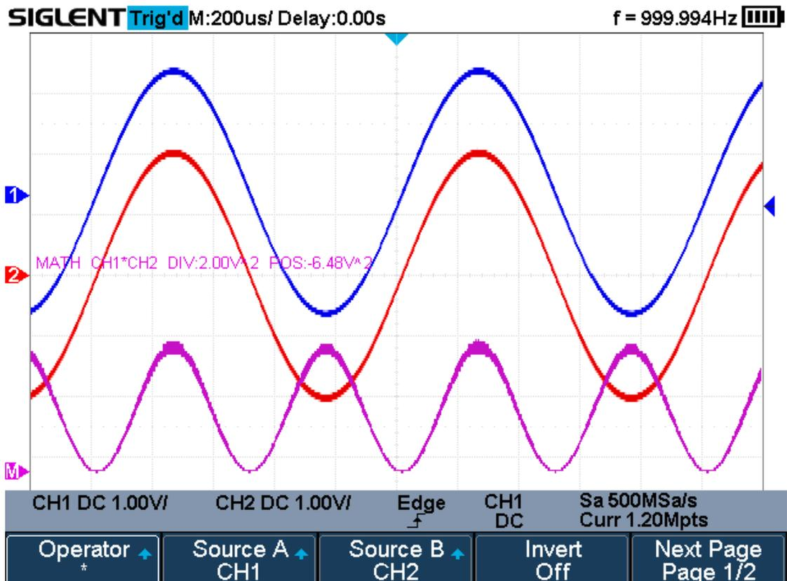
Figure 63 C1\*C2 Waveform
