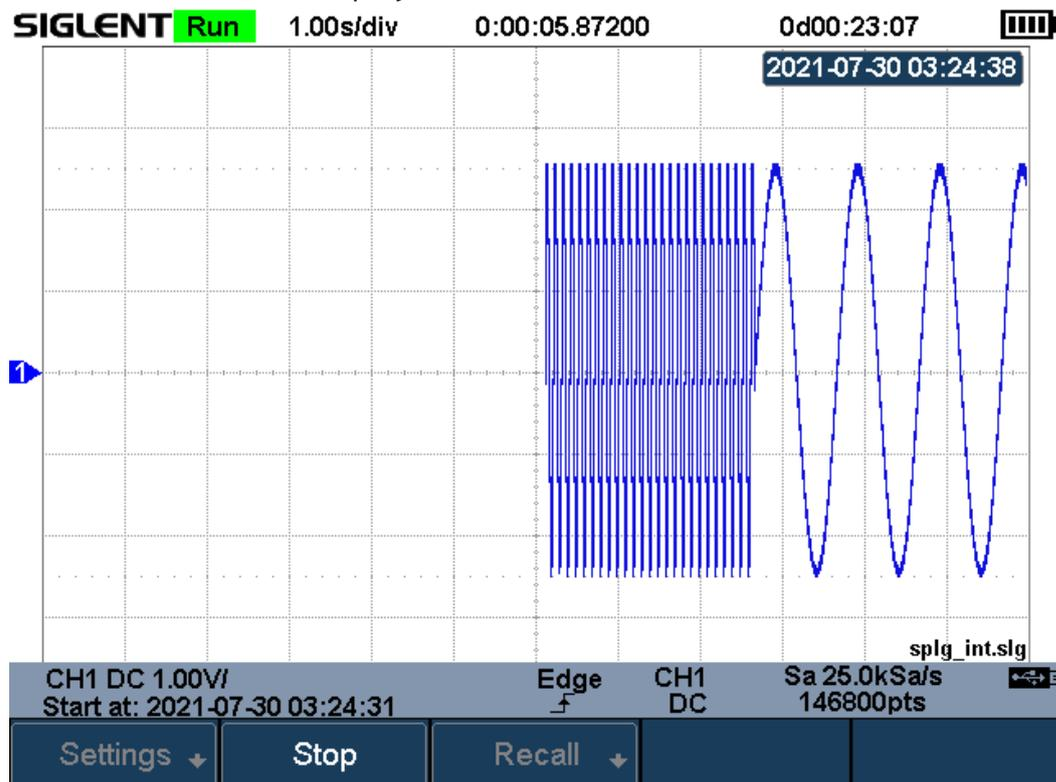
Figure 114 Start Recording Waveform
