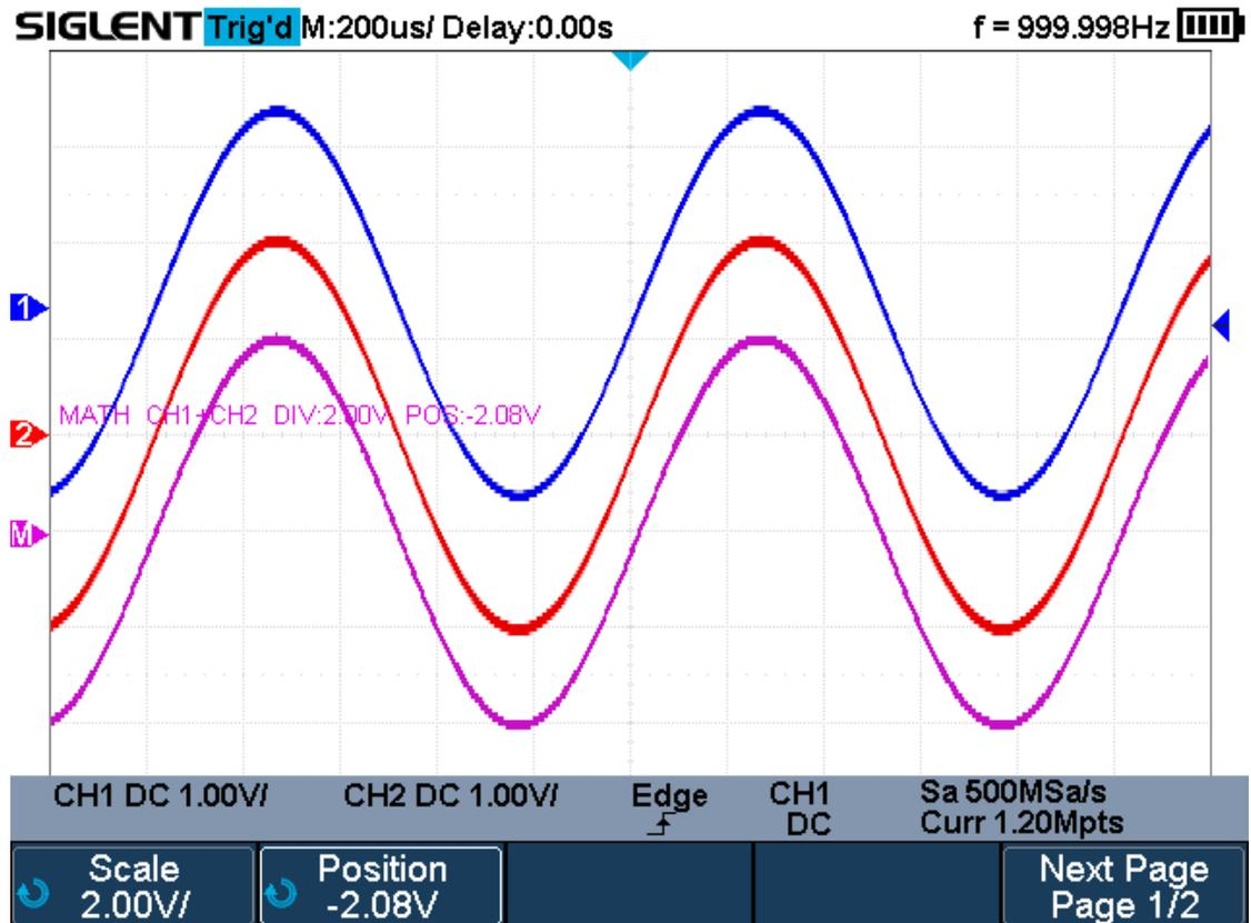
Figure 62 C1+C2 Waveform
