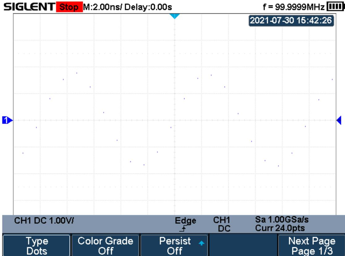
Figure 87 Dots Display
