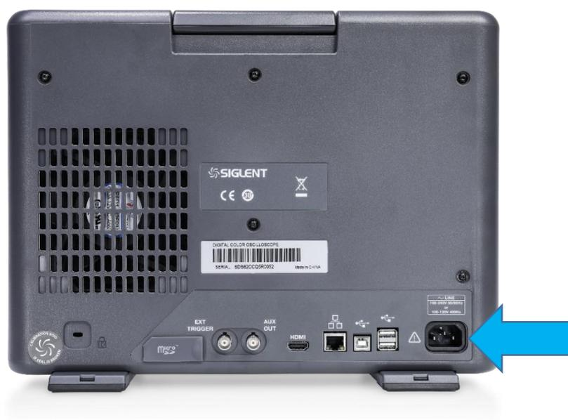
Figure 1 Connect the power cord
