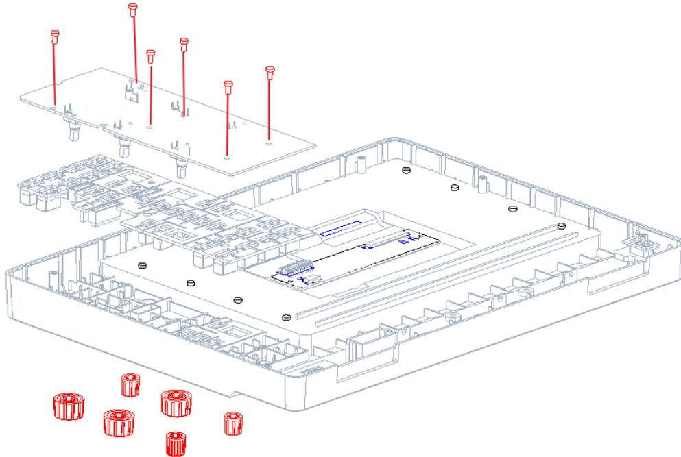
Figure 17 To remove the rubber keypad and keyboard
