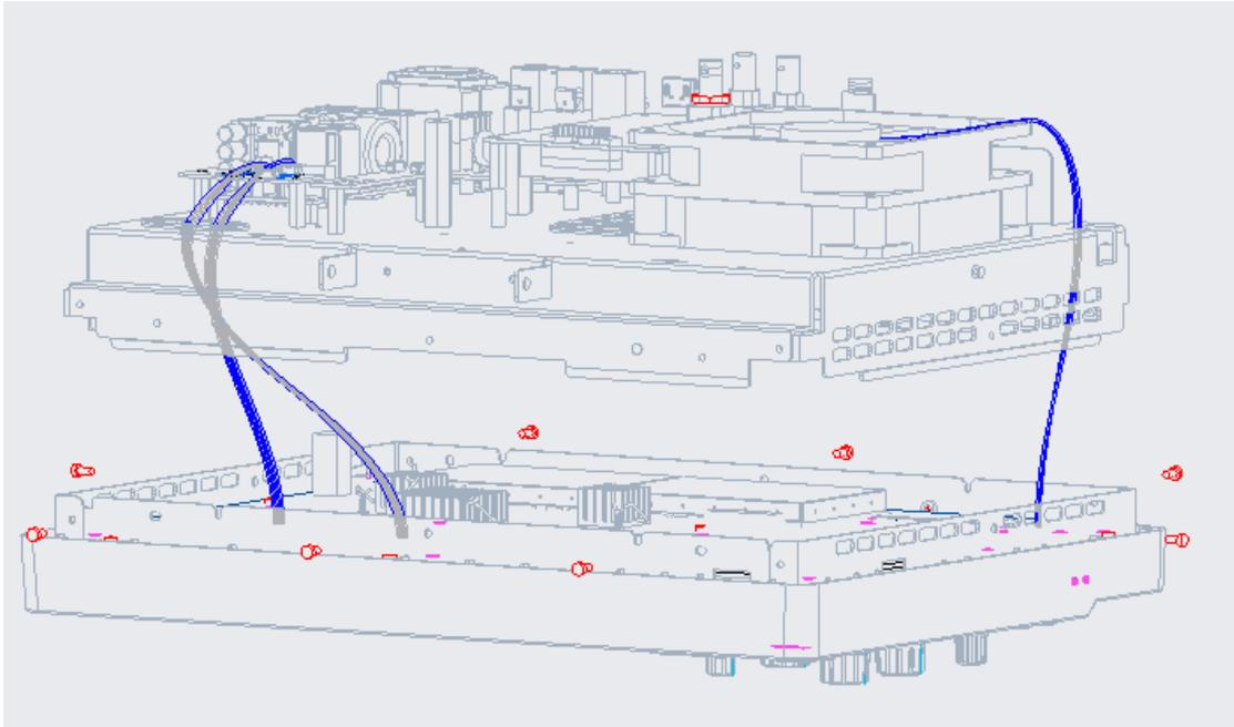
Figure 14 To remove the back panel chassis module.
