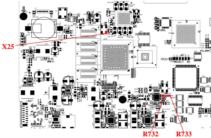
Figure 22 Test points for clock
