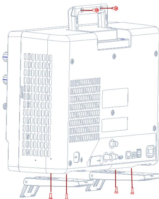
Figure 11 To remove the handle and foot
