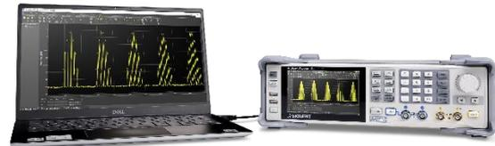
**Sequence editing and playback** The SDG7000A supports up to 1024 arbitrary wave segments, each of which can be set with a maximum of 65535 repetitions. When switching between segments, the output seamlessly moves from the last point of the previous segment to the first point of the next segment without generating an idle level. It is suitable for applications with high requirements for waveform switching.
