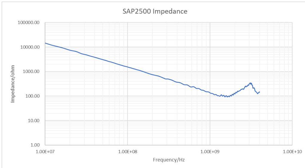
Figure 4 Input impedance over frequency of SAP2500
