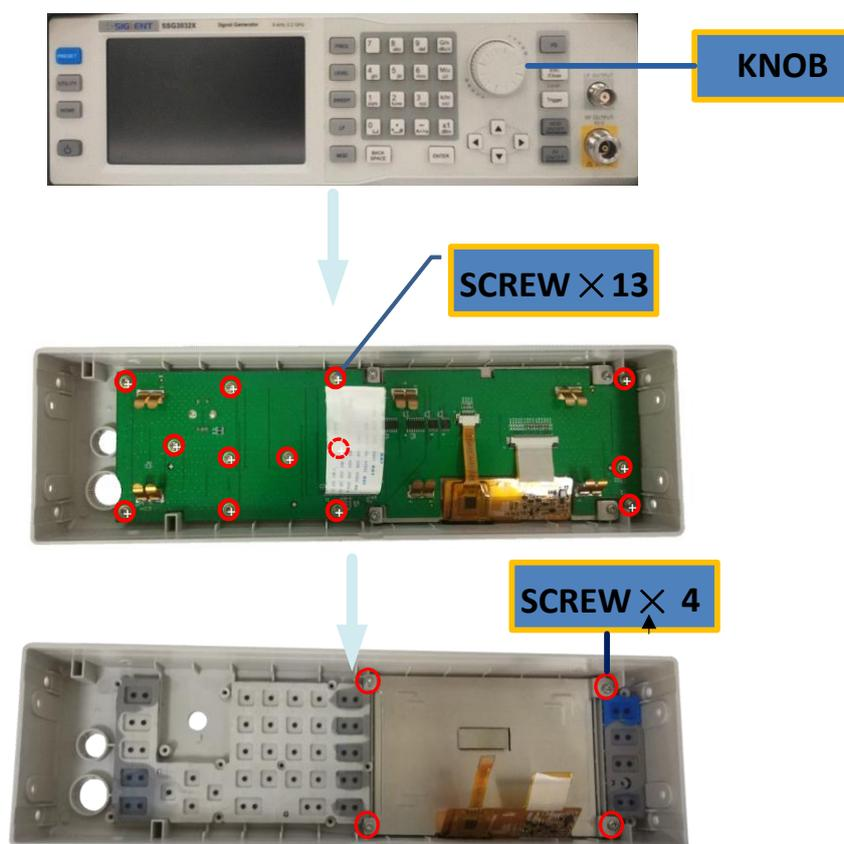
Figure 4-5 Removing the LCD and keyboard
