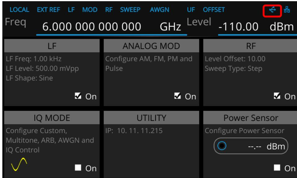
Figure 2-1 USB drive has been properly recognized
