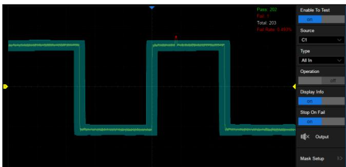
The SDS5000X utilizes a hardware-based Mask Test function, performing up to 18,000 Pass / Fail decisions each second. It is easy to generate user-defined test templates in order to provide trace mask comparisons, making it suitable for long-term signal monitoring or automated production line testing
