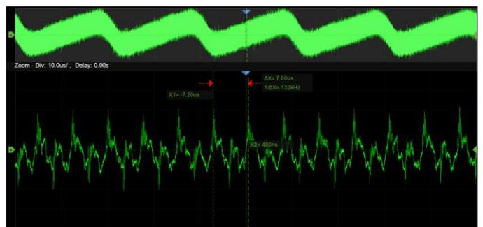
Using hardware-based Zoom technique and record length of up to 250 Mpts, users can select a slower timebase without compromising the sample rate, and then quickly zoom in to focus on the area of interest
