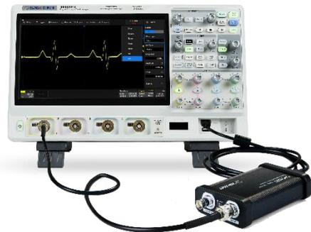
The SDS5000X can control the SAG1021I USB Function/Arbitrary waveform generator to output waveform with up to 25 MHz frequency and  $\pm 3$  V amplitude. Six basic waveforms plus multiple types of arbitrary waveforms are built-in
