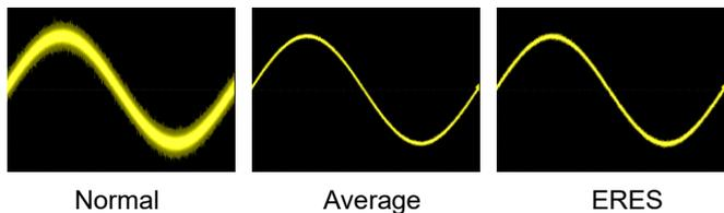
Average and ERES (Enhanced Resolution) acquisition modes are hardware-based, allowing the waveforms to be captured at a faster rate
