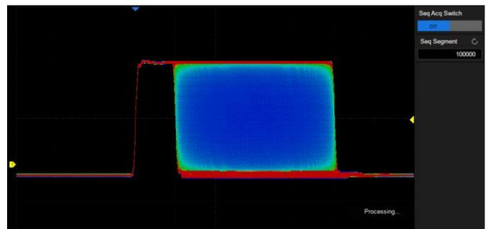
Segmented memory collection will store the waveform into multiple memory segments (up to 100,000) and each segment will store a triggered waveform as well the dead time information. The interval between segments can be as small as 2 μs. All of the segments can be played back using the History function
