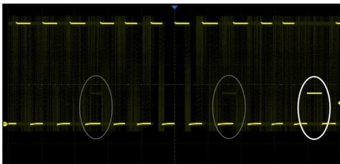
With a waveform update rate of up to 110,000 wfms/s, the oscilloscope can easily capture unusual or low-probability events. In Sequence mode the waveform capture rate can reach 500,000 wfms/s
