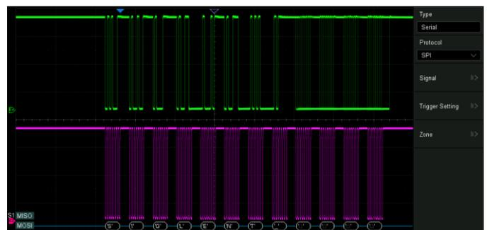
Display the decoded characters through the events list. Bus protocol information can be quickly and intuitively displayed in tabular form. I<sup>2</sup>C, SPI, UART, CAN, LIN, CAN FD, FlexRay, I<sup>2</sup>S, MIL-STD-1553B, SENT, Manchester and ARINC 429 are supported
