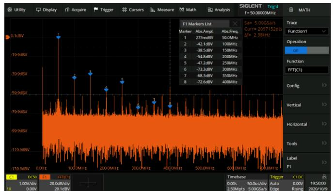
Hardware accelerated FFT supports up to 2 Mpts operation. This provides high frequency resolution with a fast refresh rate. The FFT function also supports a variety of window functions so that it can adapt to different spectrum measurement needs. Three modes (Normal, Average and Max hold) can satisfy different requirements for observing the power spectrum. Auto peak detection and markers are supported
