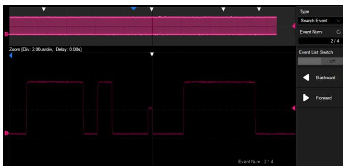
The SDS5000X can search events specified by the user in a frame. Events flagged by the Search can be recalled automatically using Navigate. It can also navigate by time (delay position) and history frames
