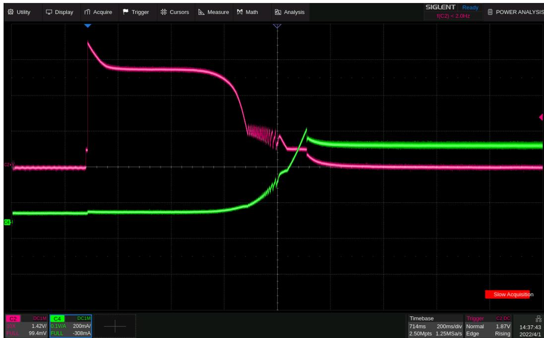
Voltage and current waveforms on the MOSFET at power-up
