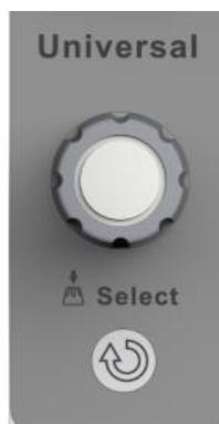
When the parameter setting area is highlighted, the Universal Knob can be used to adjust the parameter. Press the knob to select an option from the list. The default function of the Universal Knob is to adjust the intensity of the waveform traces.
