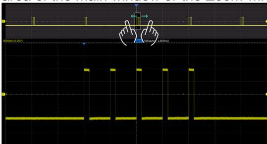
Adjust the horizontal/vertical scale of the main window by using a pinching or spreading gesture in the gray area of the main window.
