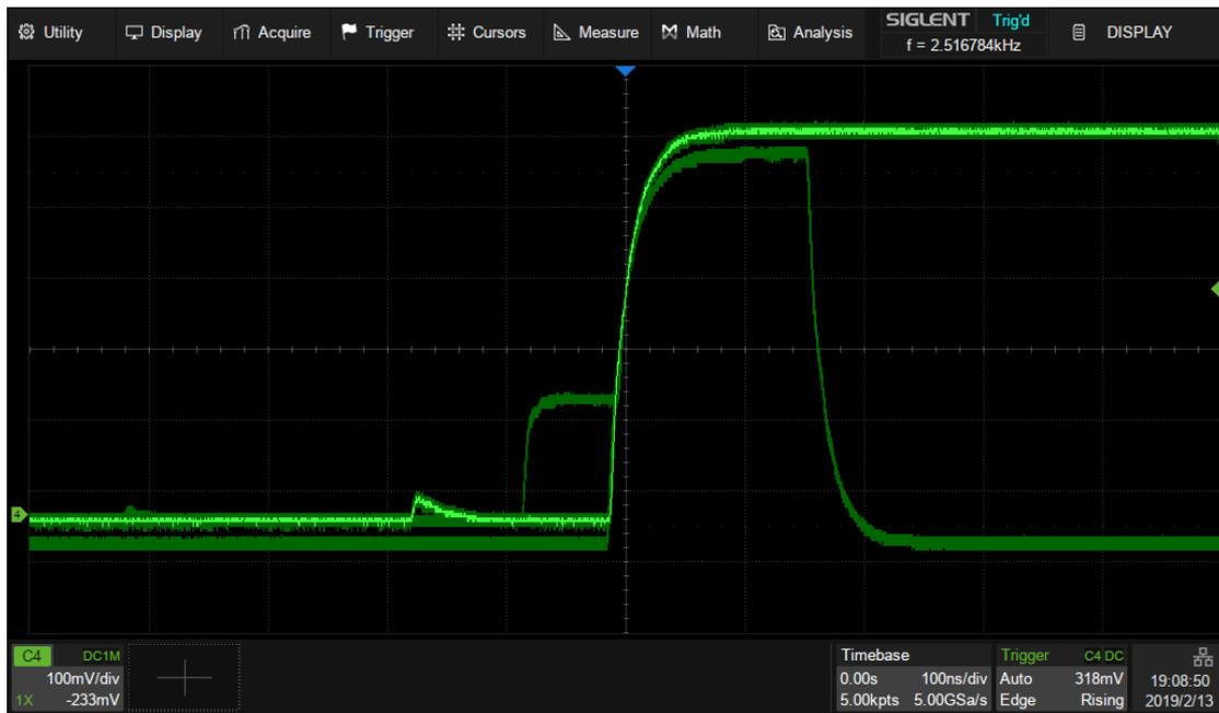
In this case zone trigger is a quick and simple way to capture the waveform. Enable the zone trigger, and draw a box to intersect with the bus contention part, as shown in the figure below:
