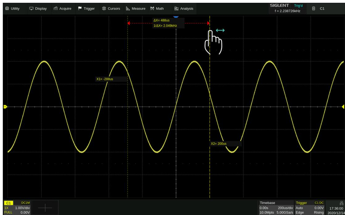
Touch the display area of  $\Delta X$  (or  $\Delta Y$ ) in M1 mode and drag it to move the two cursors simultaneously, as shown in the figure below. This is equivalent to the operation on the cursor type X1-X2 or Y1-Y2.
