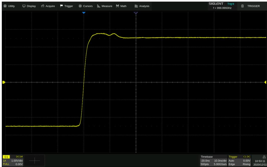
Timebase = 10 ns/div, Horizontal Delay = -20 ns = - 2 div
