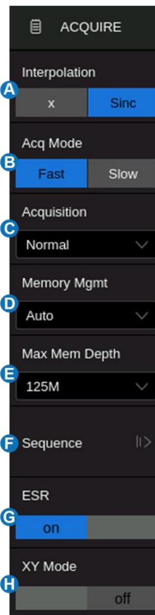
**Interpolation** -- At small timebase settings, the number of original points on the screen may be less than the number of display pixels in the grid area, so
