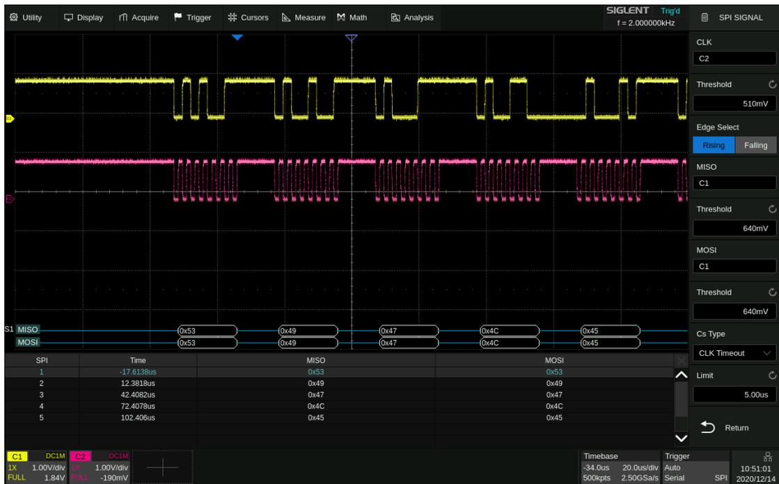
If the data width is set to be greater than 8 bits (such as 16 bits), measure the clock idle time between 8-bit data packets as 11.28 us, and then set the timeout time to a value between 11.28 and 150 us. In this example, it is set to 20 us:
