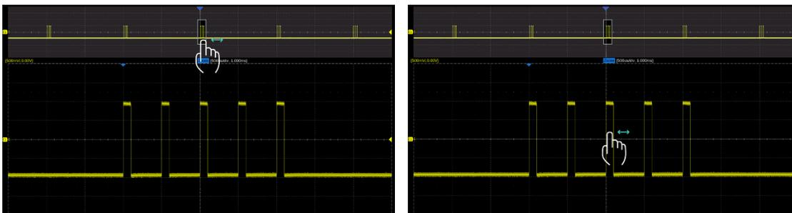
Adjust the horizontal position of the zoom area by dragging left and right in the zoom area of the main window or waveform in the Zoom window.
