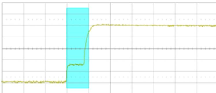
With a simple edge trigger, it is unlikely to trigger consistently on this anomaly. Thanks to the high waveform update rate of the SDS6000A, we can confirm there is bus contention happening by enabling the persistence display, as shown in the figure below:
