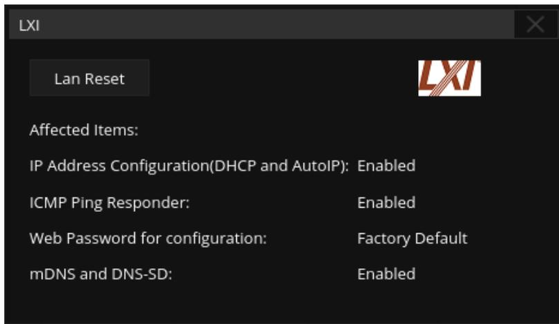
Touch **LAN Reset** to restore the LAN defaults to your oscilloscope. It will enable automatic IP, ICMP Ping responder, and Multicast DNS, and reset the webserver password which is set in **Utility > I/O > Web Server**.
