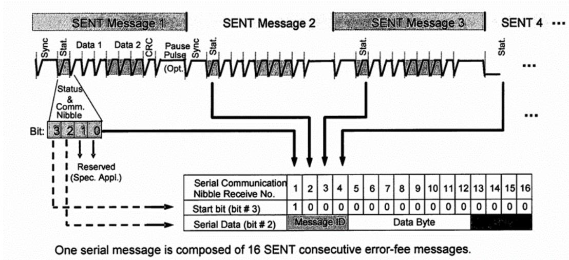
The serial message frame contains 21 bits of payload data. Two different configurations can be chosen determined by the configuration bit (serial data bit #3, serial communication nibble No. 8):
