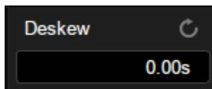
**Virtual Keypad:** Sets parameters with a numerical value. Touch the parameter region, and the parameter can be adjusted by the universal knob on the front panel or by the mouse wheel; touch the region again, then the virtual keypad appears:
