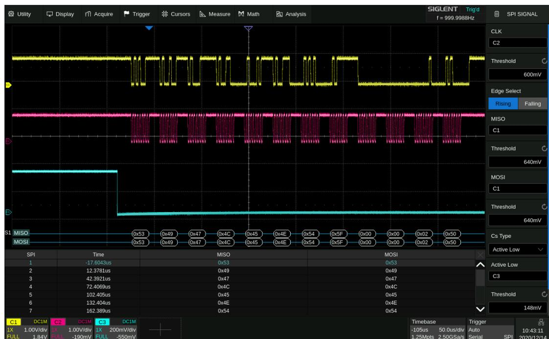
When the CS type is set to Clock Timeout, turn on Cursor, measure the clock idle time between frames as 150  $\mu$ s, and measure the interval between clock pulses as 1.28  $\mu$ s, then set the timeout to a value between 1.28  $\mu$ s and 150  $\mu$ s. In this example it is set to 5  $\mu$ s:
