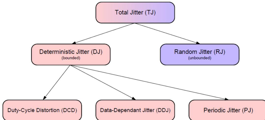
Figure 31.1 Jitter decomposition tree
