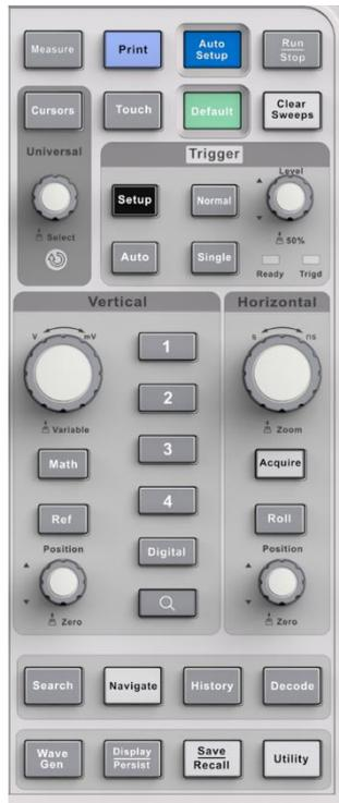
The front panel is designed to operate the basic functions without having to open the software menu. Most of the front panel controls duplicate functionality available through the touch screen display but the operation is more quickly achieved.
