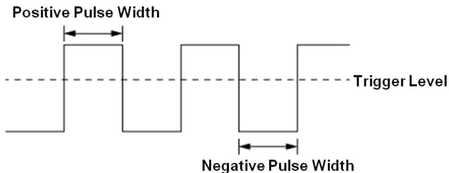
**Less than a time value ( $\leq$ )** -- Trigger when the positive or negative pulse time of the input signal is lower than the specified time value. Below is an example of a trigger condition set to a positive pulse width  $< 100\text{ns}$
