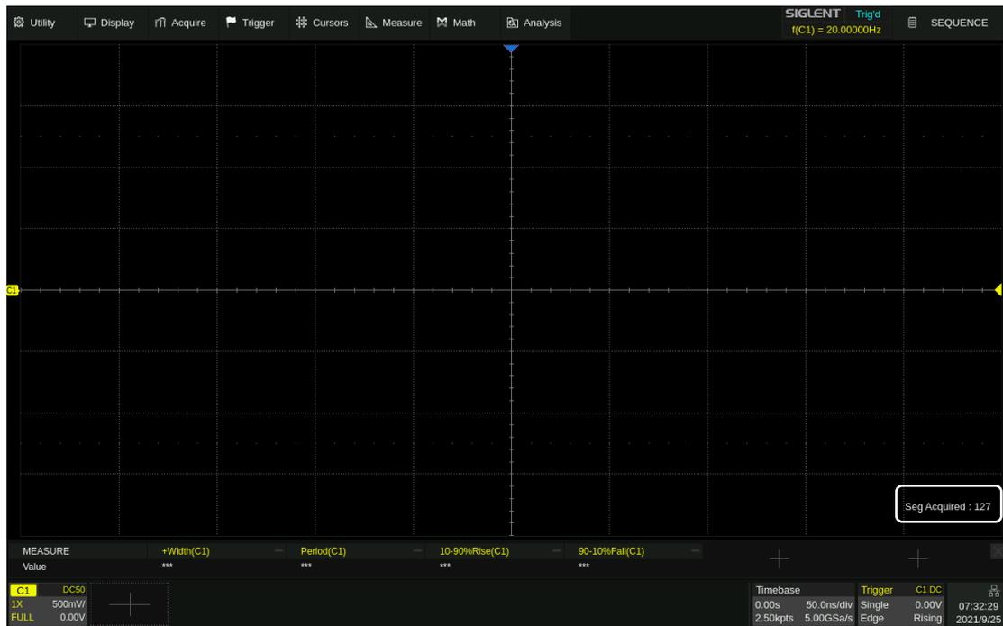
In Sequence mode, there is no waveform displayed on the screen until the acquisition is completed. During acquisition, there is a counter on the screen indicating the number of segments that have been acquired.
