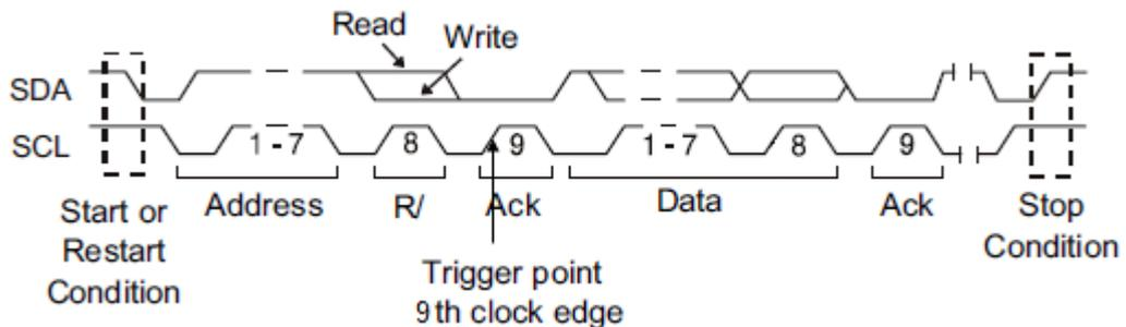
Frame (Start: 7-bit address: R/W: Ack: Data: Ack: Data2)—If all bits match, then trigger on the Ack bit followed by the Data2.
