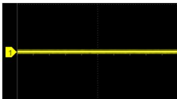
**Channel Offset Indicator** with a channel number shows the offset position of the corresponding channel.
