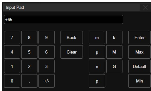
Let's use the operation of setting the "deskew" of a channel as an example: If the expected value is 65 ns, input "65" on the virtual keypad, and then choose *n* as the unit "ns" to complete the operation. On the virtual keypad, touching the button *Max*, *Min*, and *Default* quickly sets the parameter to the maximum, minimum, and default values.
