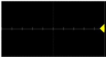
**Trigger Level Indicator** shows the level where the waveform triggers on the vertical axis.
