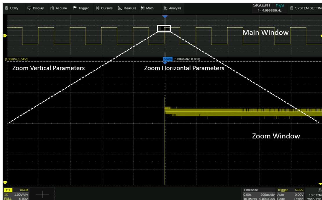
The area not covered by the gray background in the main waveform area is the range to be zoomed in (zoom area). Touch the Zoom Vertical Parameters and Zoom Horizontal Parameters regions shown in the figure above to recall the quick dialogs for setting the vertical and horizontal parameters of the zoom window.
