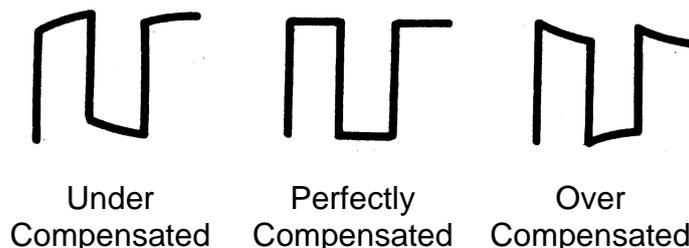
5. Use a non-metallic driver to adjust the low-frequency compensation
