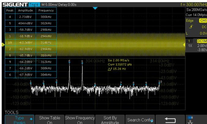
The math co-processor enables FFT analysis of incoming signals using up to 128k samples per waveform. This provides high frequency resolution with a fast refresh rate. The FFT function also supports a variety of window functions so that it can adapt to different spectrum measurement needs. It also supports Peaks, Markers, a variety of FFT points.
