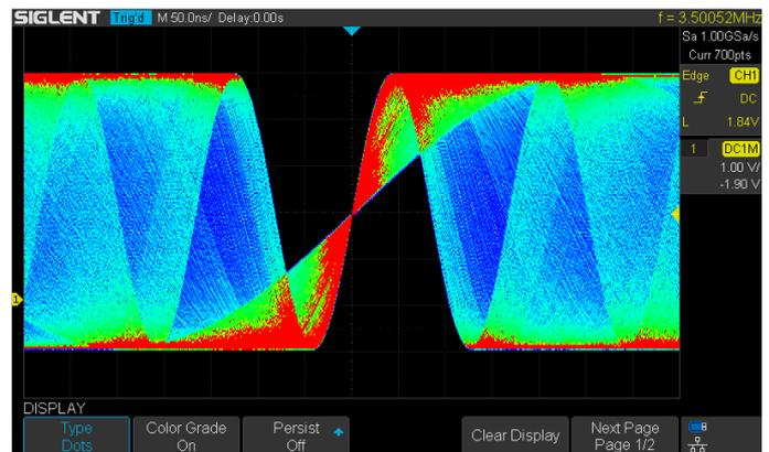
The color temperature display is similar to the intensity-graded trace function, but the trace occurrence is represented by different colors (color "temperature") as opposed to changes in the intensity of one color. Red colors represent events that occur more frequently, while blue is used to mark points that occur less frequently.
