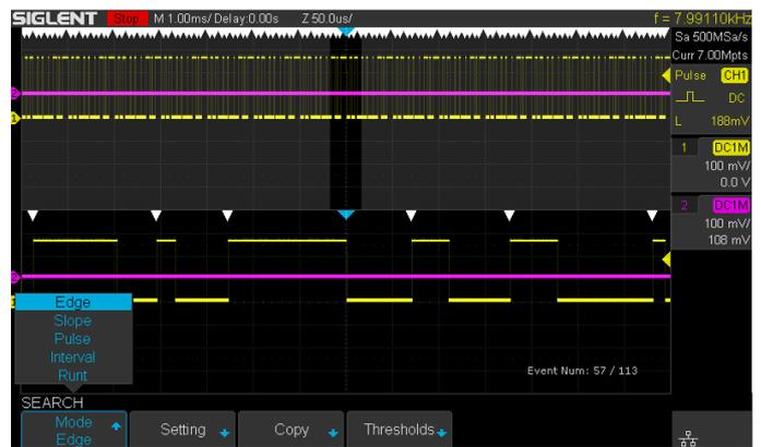
The SDS1000X-U can search events specified by the user in a frame. It can also navigate by time (delay position) and historical frames.
