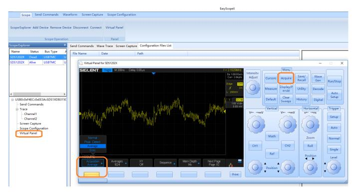
5. Select Waveform, and use the Play/Pause button to acquire the waveform of interest. Then, select Save > select the channel of interest > select the type of CSV to save > Press Save to open a file dialog box.
