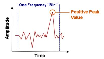
Positive peak detectors are the most commonly used detector type. They are perfect for measuring the peak power of a signal as well as determining the "worst case" signal in EMI applications.
