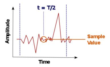
This detector type is applicable to noise, noise-like signals, or small amplitude continuous wave (CW) signals that are near the noise floor of the analyzer.
