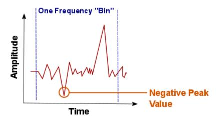
Negative peak detectors are rarely used, but can be helpful when comparing positive and negative peak values when looking for CW and Pulsed signals. CW signals will have less difference between positive and negative peak values for a given frequency bin. A pulsed signal could have a significant difference
