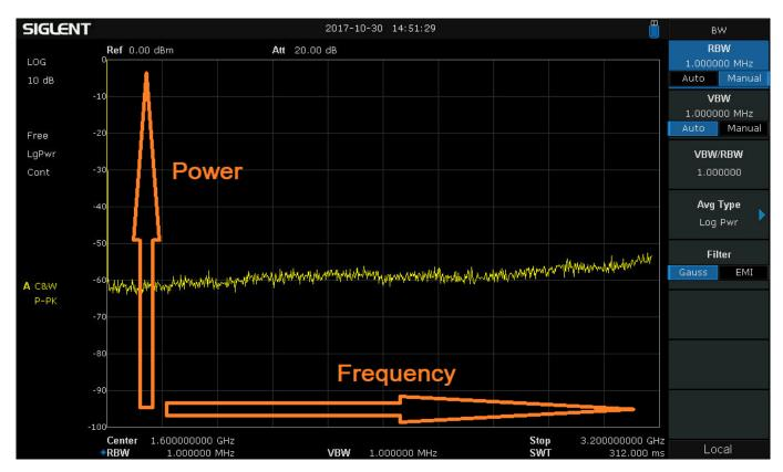
The horizontal span (which composes a frequency span when the instrument is configured to sweep/not in zero span mode) is comprised of 751 discrete samples (also called "bins").
