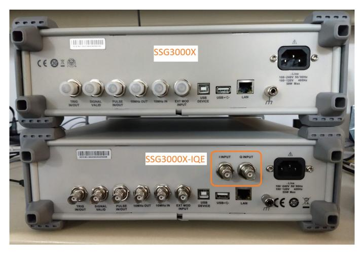
NOTE: The -IQE version features I and Q inputs and associated hardware not included with the SSG3000X version.
