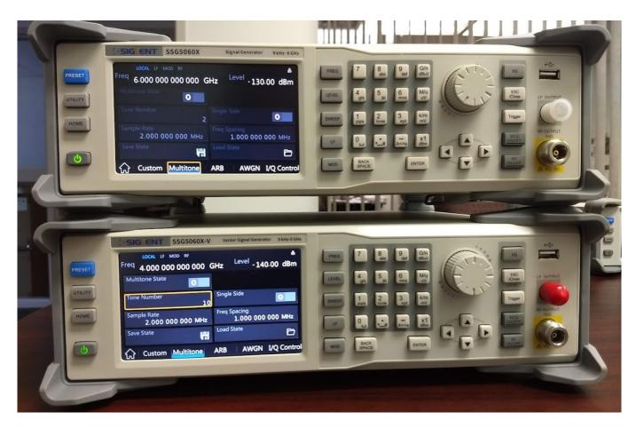
NOTE: The -V version features I and Q inputs and associated hardware not included with the SSG5000X version. The front panel/GUI of both does include the multitone menu, but it is greyed out/non-operational on SSG5000X versions.
