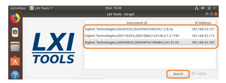
• **SCPI command line:** Send instrument specific commands. Click on the instrument you wish to communicate with and then enter the command. For queries (commands that require an instrument response, or read function), the returned string will be shown in the text box:
