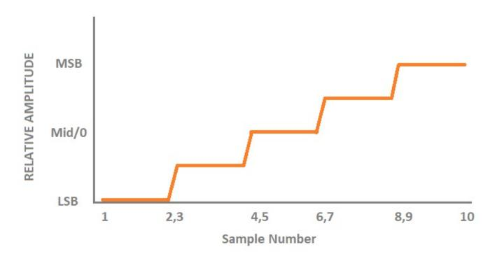
The SDG waveform data requires each sample to first be formatted as binary, little-endian, 2's complement. For easier human viewing, the example enters the data in hex format and then "unhexes" the data before it is added to the command string which is then sent to the instrument.
