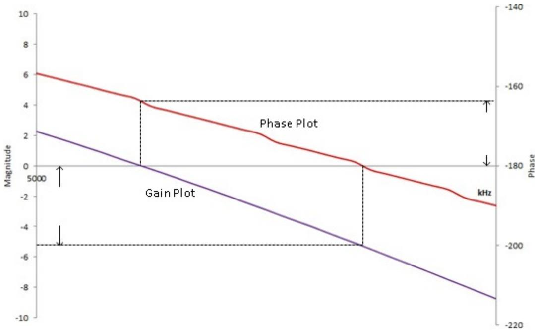
Figure 3: Bode Plot, phase, and gain margin
