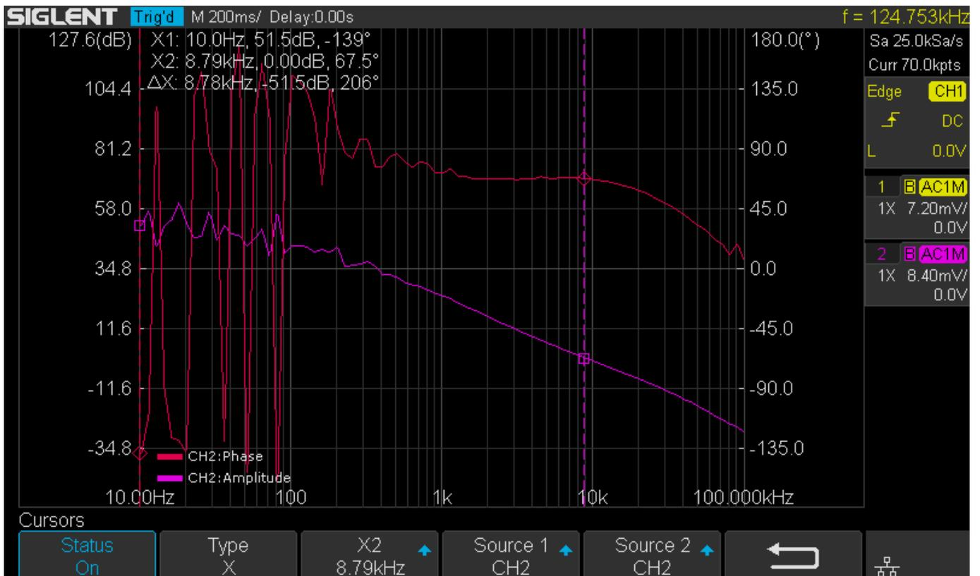
Figure 12: Cursor measurement on the Bode plot
