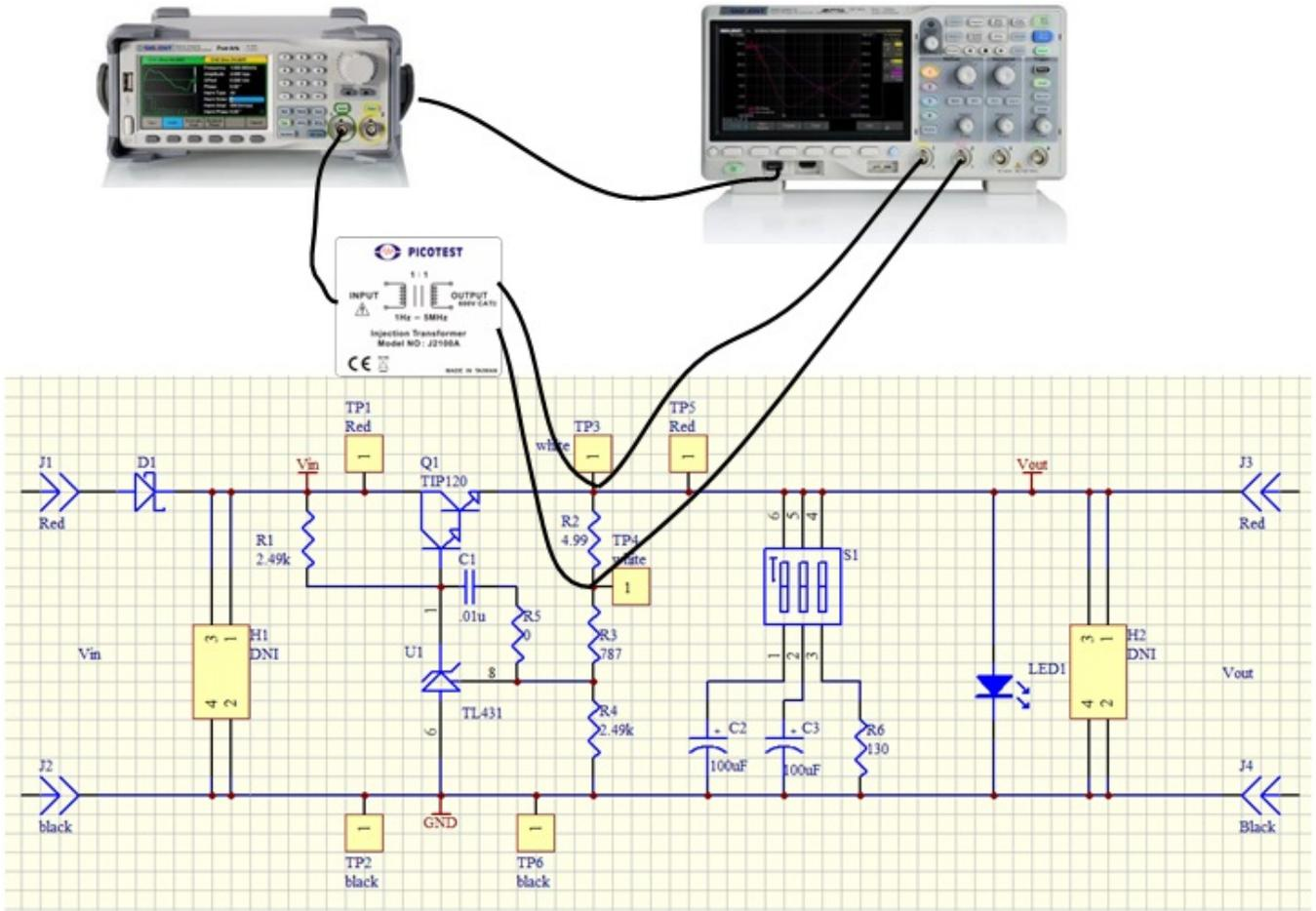
Figure 8: Circuit connection
