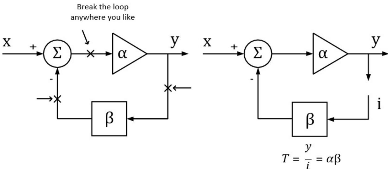
Figure 4: Breaking the loop in a typical feedback system
