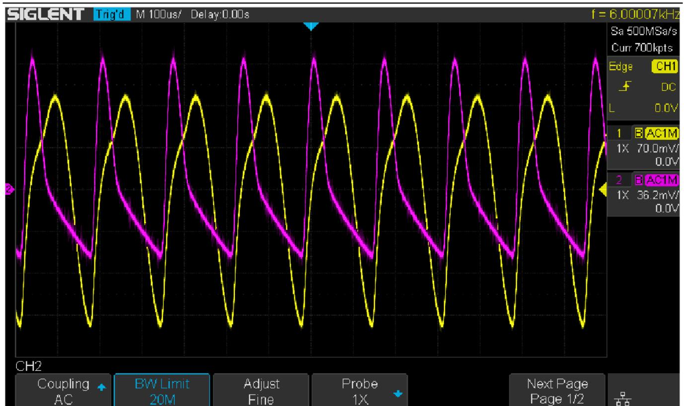
Figure 15: Distortion in the time domain
