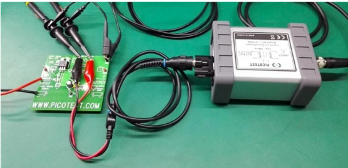
Figure 9: Probe and Transformer connections to the DUT
