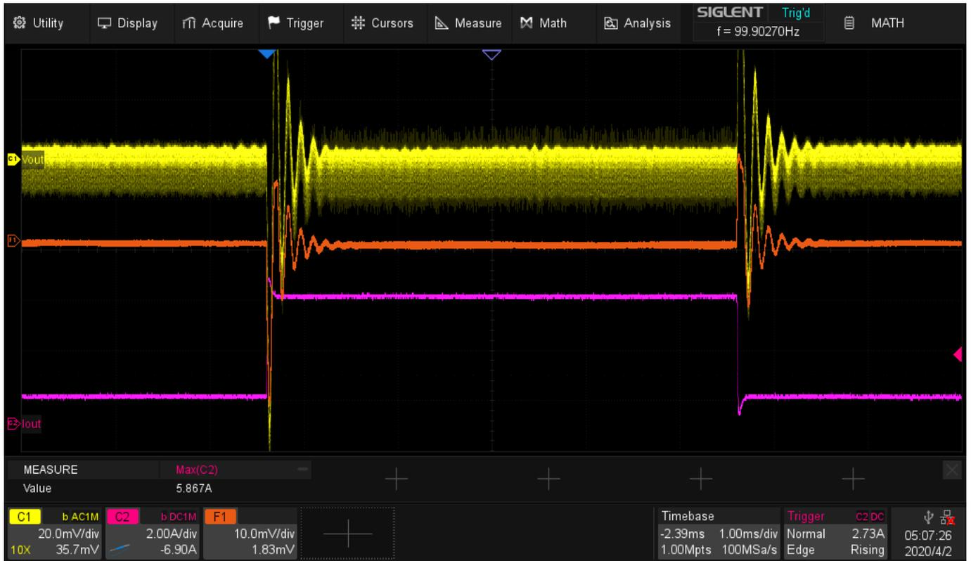
The scaling on these two images is exactly the same. You can see a large amount of ringing associated with the detuned supply. This design is very close to becoming an oscillator with this load. If our step duration was any shorter, the supply voltage wouldn't be settled and our output would be very poorly regulated.
