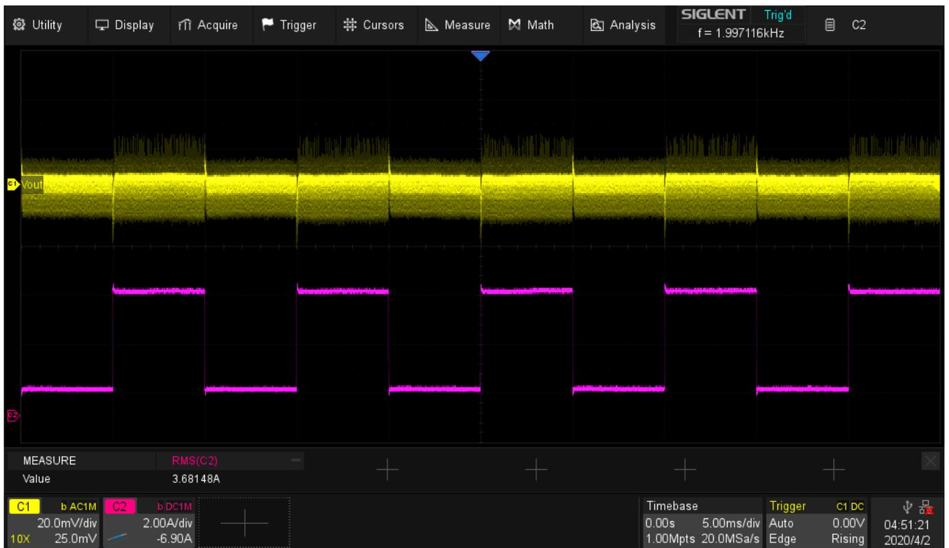
Verify that the supply high and low current values match the setpoints. For this example, we have 1 A for 5 ms and 5 A for 5 ms.. which is what we observe.
