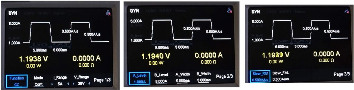
This will continuously cycle from 1 A for 5 ms to 5 A for 5 ms with 500 mA/us slew rate.
