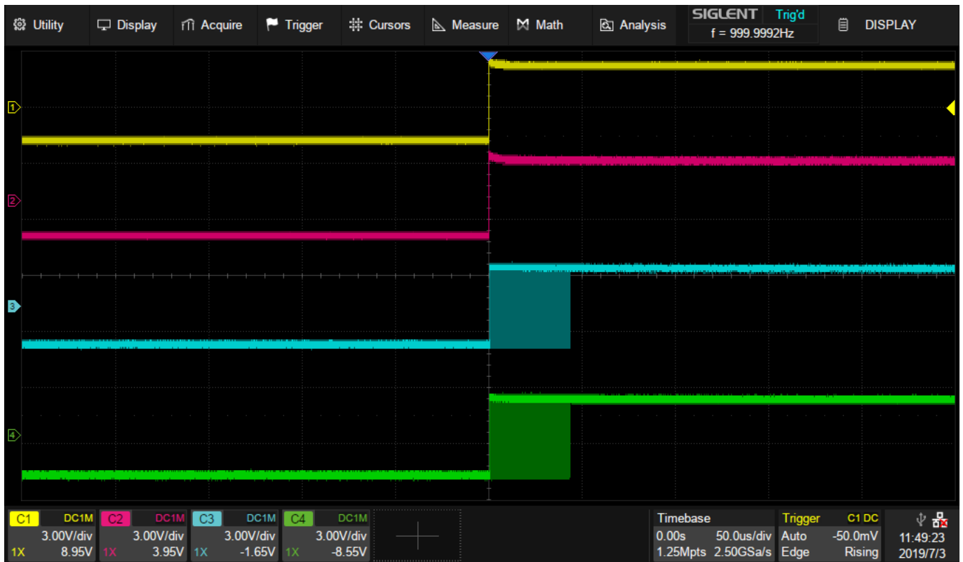
Figure 4. Four signals phase drift without synchronization
