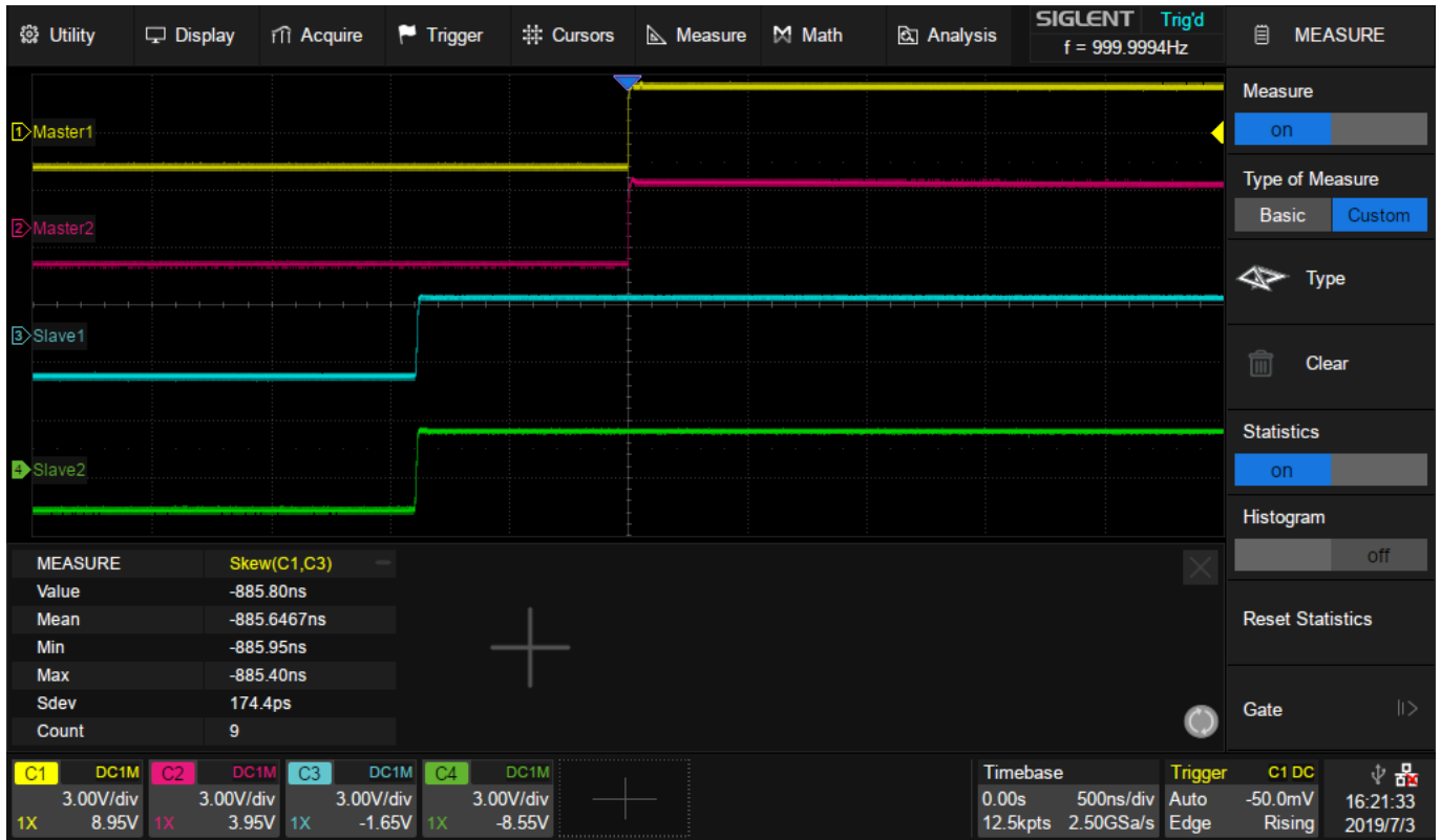
Figure 9. Measure the Skew between Master and Slave Devices
