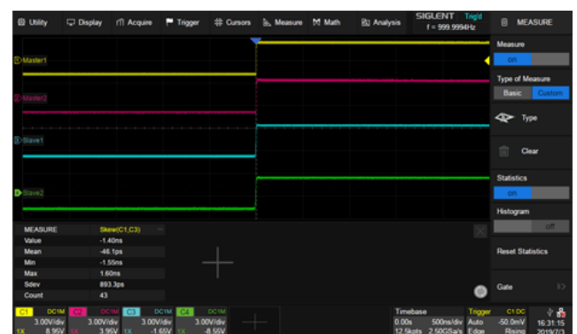
Figure 10. Eliminate the Slave Delay
