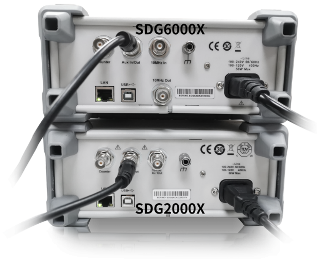
Figure 2. Connect SDG2000X and SDG6000X Aux In/Out
