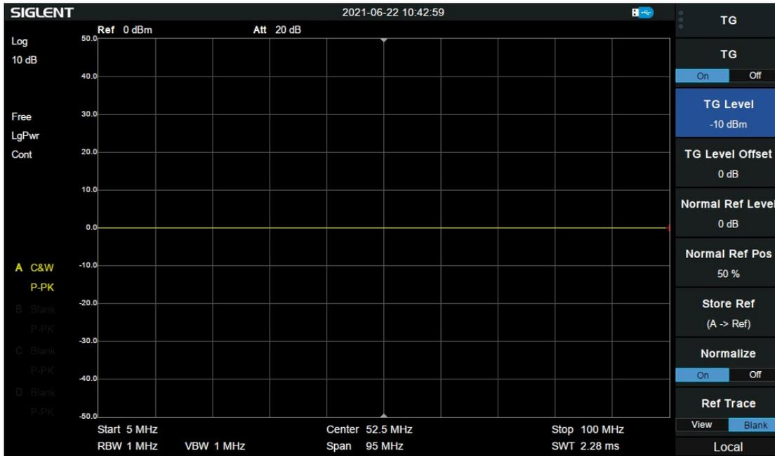
7. Press Norm Ref Pos -> 90%. This will allow for a convenient location on the spectrum analyzer screen to observe the filter's frequency response curve.
