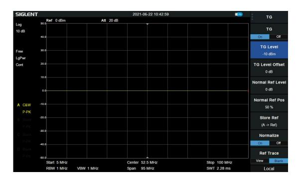
7. Press Norm Ref Pos -> 90%. This will allow for a convenient location on the spectrum analyzer screen to observe the filter's frequency response curve.
