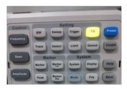
4. Enter an appropriate tracking generator output power. For example, -10 dBm. Press TG level-> -10 -> dBm.
