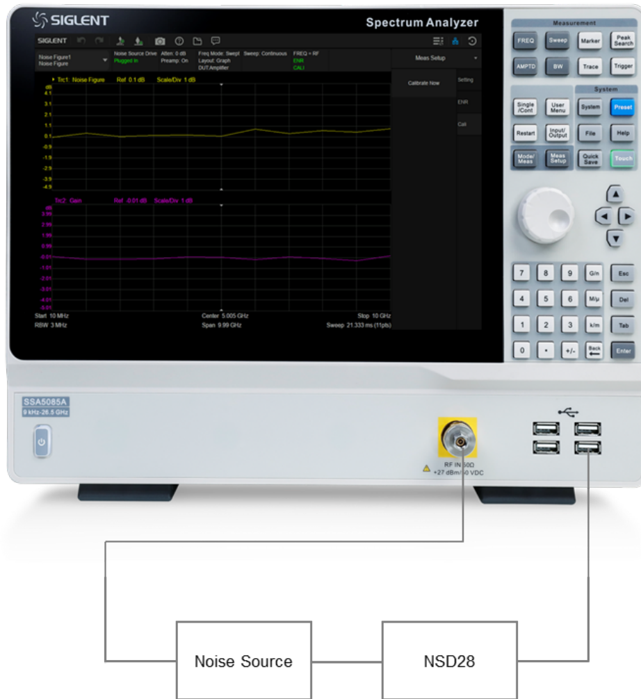
Figure 1-2 Connection setting of noise figure measurement calibration
