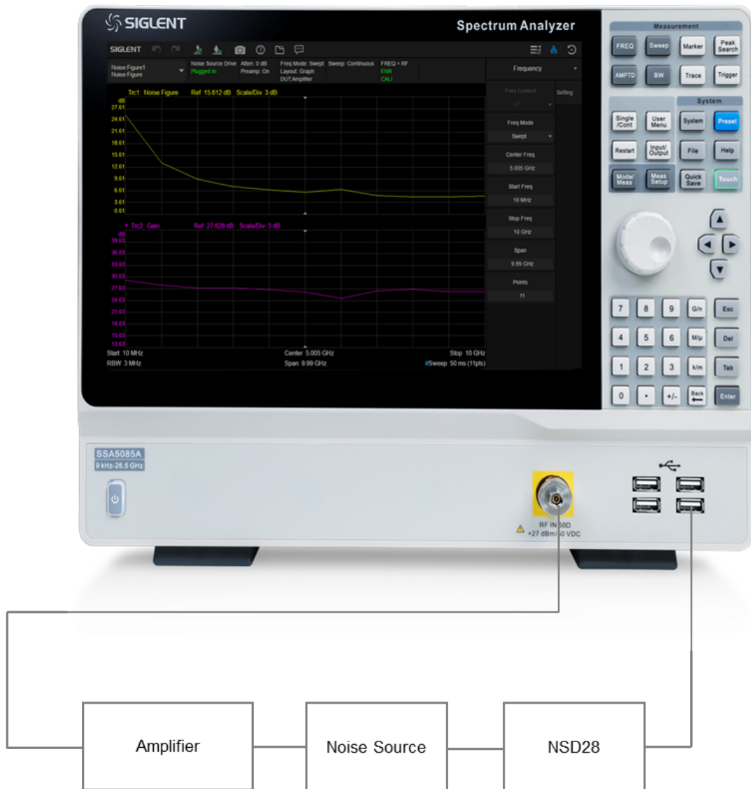
Figure 1-6 Connection settings for noise figure measurement
