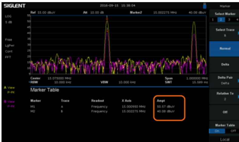
Figure 5: Comparison of two scans using the marker table function of the SIGLENT SSA3000X spectrum analyzer. The Yellow trace was collected without attenuation while the Pink trace was collected after adding a 10 dB external attenuator.
