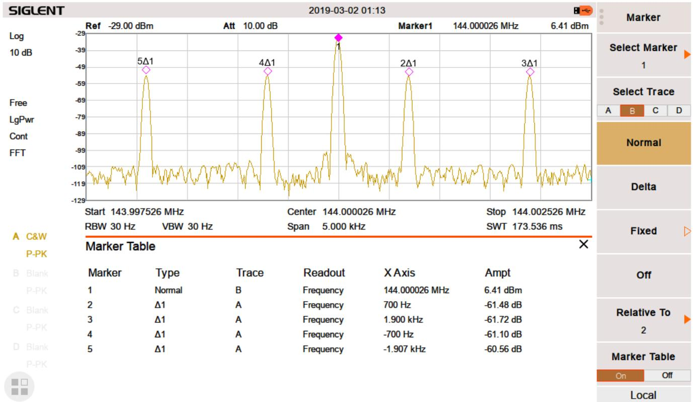
Here, you can see the carrier at 144 MHz, and the two tones at +700, +1900, -700, and +1900 Hz from the carrier.. as expected.
