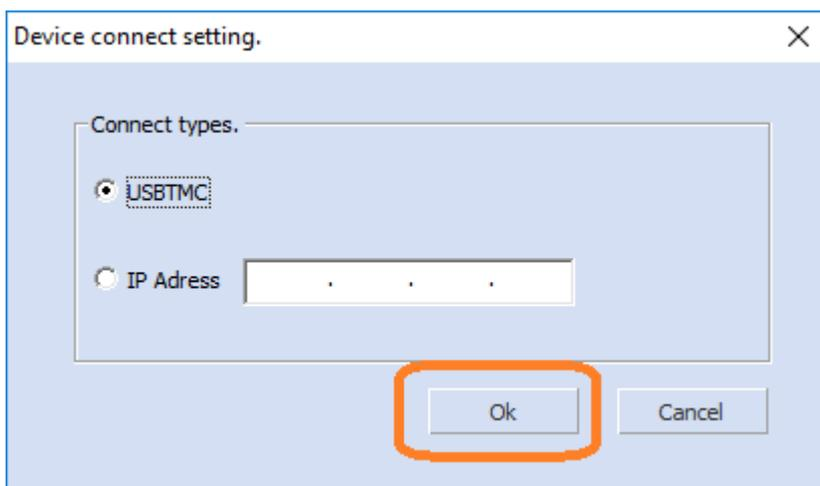
7. Select the correct USB device, Waveform Name, and Channel.. press OK:
