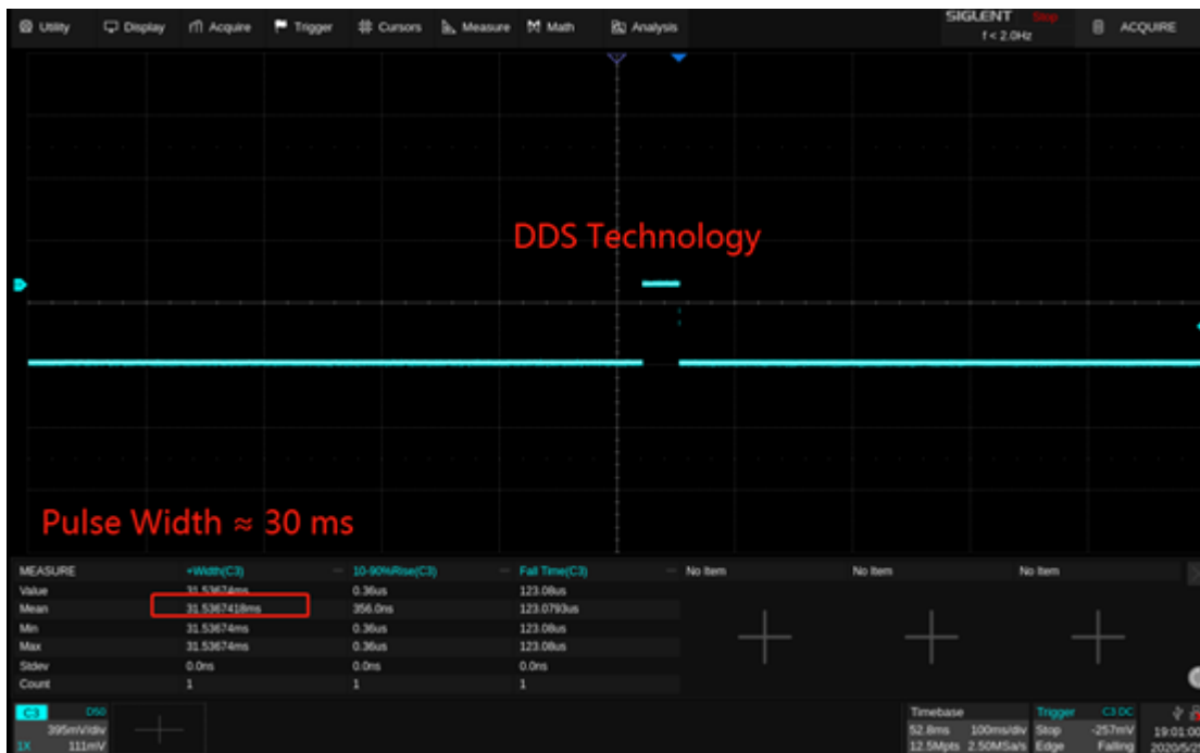
Figure 6: 1 Hz pulse signal generated by DDS
