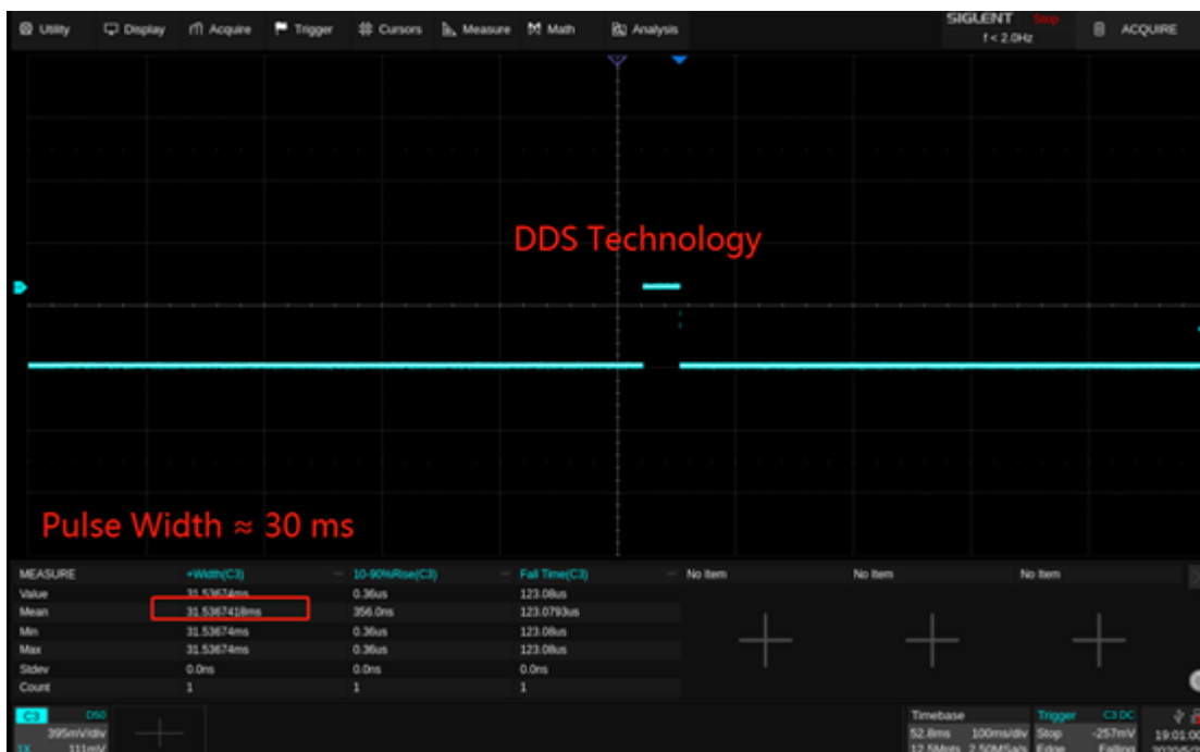
Figure 6: 1 Hz pulse signal generated by DDS
