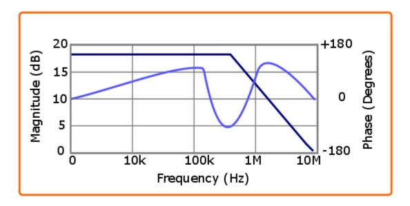
By showing both the magnitude and phase information on the same graph, you can evaluate some of the tested device's basic qualities. A function generator and oscilloscope can be used to manually collect and compare the phase and amplitude data for a given device, but this can be tedious and time-consuming.
