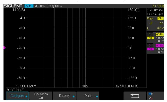
3. Press AWG to set the signal amplitude and set the expected device load impedance. Press the back arrow to return to the Configure screen.
