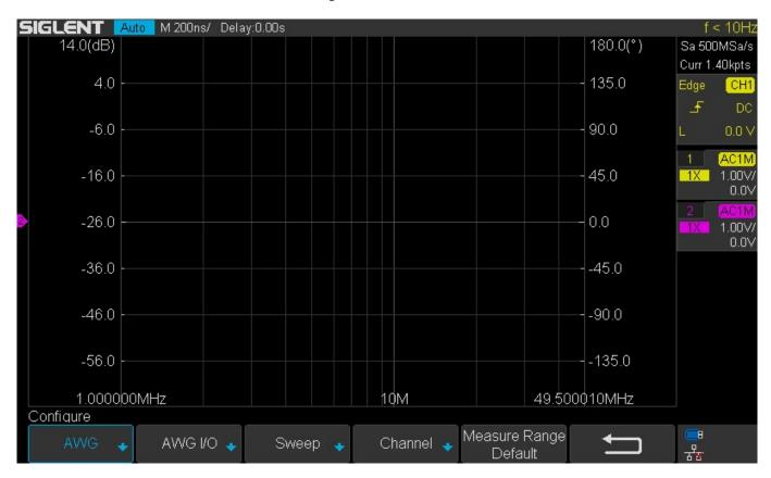
7. Now, confirm the channel connections by pressing Channel:
