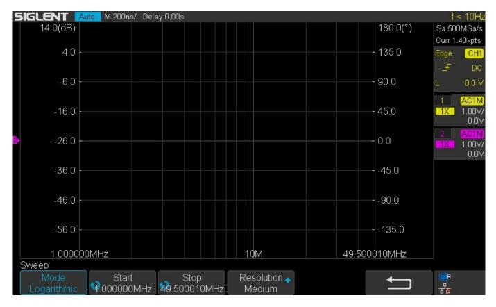
To set the Start and Stop frequencies, press the appropriate soft key (Start or Stop).
