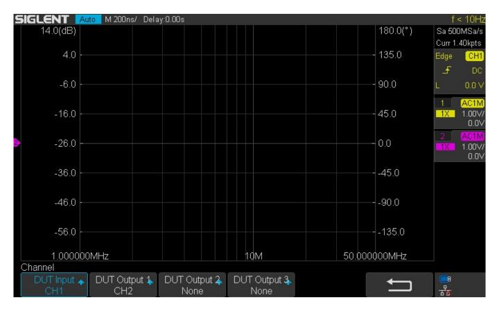
Here, you can see we have DUT input (the direct signal from the generator) connected to Oscilloscope channel 1. The scope CH2 is connected to the DUT output (the through connection).
