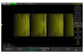
The measurement Logger is designed to collect measurement values for a long time. The data is logged in memory. After logging is complete, the data can be saved into the internal flash or external U disk.
