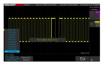
The Sample Logger is the mode of logging the sampling points over long time durations. . Data is logged into the internal flash or external U disk in real time. After logging is complete, the user can recall the sampling points on the oscilloscope, or analyze the saved data on the computer.
