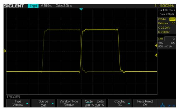
Figure 28 Relative Window Trigger
