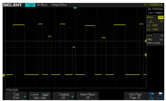
Figure 32 Runt Trigger
