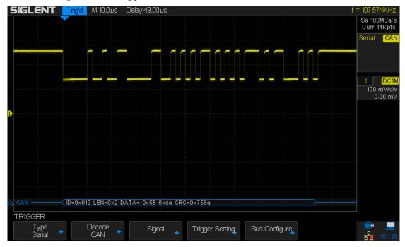
Figure 56 CAN Trigger
