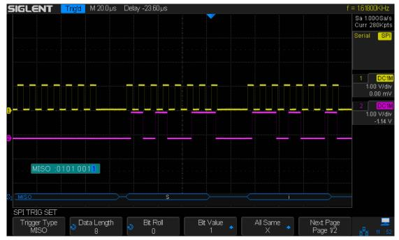
Figure 48 SPI Trigger
