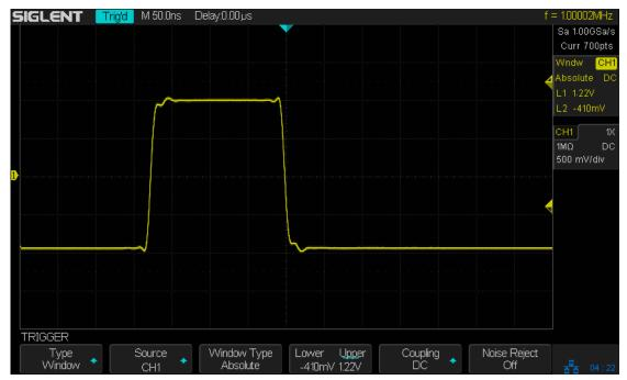
Figure 27 Absolute Window Trigger
