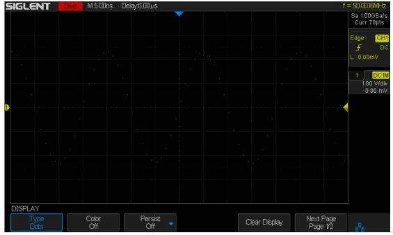
Figure 59 Dots Display
