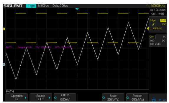
Figure 48 Integral with Offset
