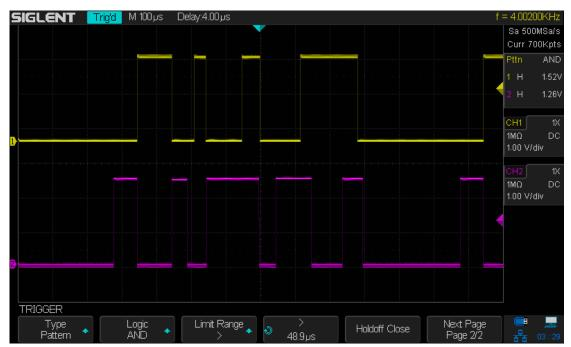
Figure 33 Pattern Trigger
