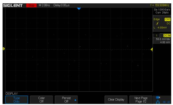
Figure 11 Display Type Set to Dots
