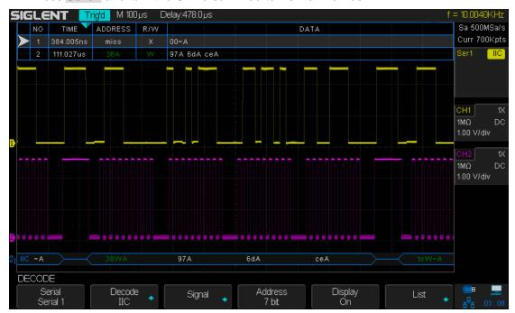
Figure 42 IIC Decode Result
